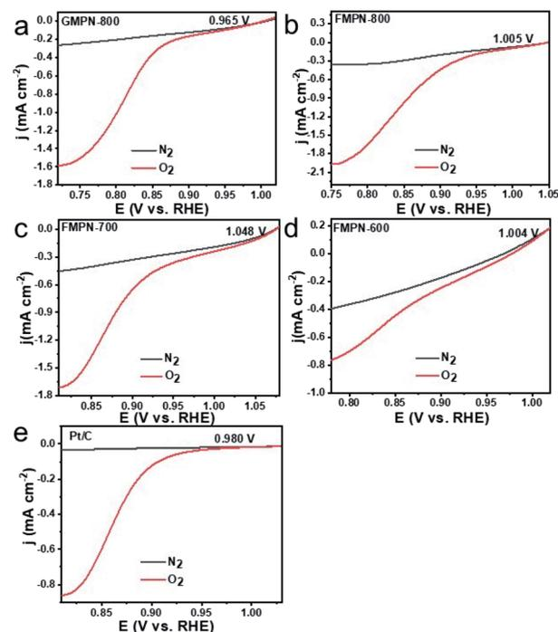
Fig. 4 LSV curves of (a) GMPN-800, (b) FMPN-800, (c) FMPN-700 and (d) FMPN-600 and (e) Pt/C electrodes in 0.1 M KOH solution saturated with N<sub>2</sub> and O<sub>2</sub> at a scanning rate of 5 mV s<sup>-1</sup>.
