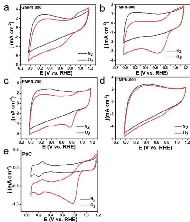
Fig. 3 CV curves of GMPN-800 (a), FMPN-800 (b), FMPN-700 (c), FMPN-600 (d) and commercial Pt/C (e) samples at a scan rate of 20 mV s<sup>-1</sup> in the N<sub>2</sub> and O<sub>2</sub>-saturated KOH solution.
