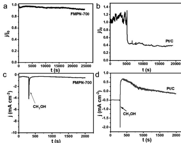
Fig. 5 Chronoamperometric responses of (a and c) FMPN-700 and (b and d) Pt/C electrodes at  $-0.35 \text{ V}$  (vs. Ag/AgCl) in  $\text{O}_2$ -saturated  $0.1 \text{ M}$  KOH solution and  $0.1 \text{ M}$  KOH solution injected with methanol ( $3 \text{ M}$ ) during ORR process.
