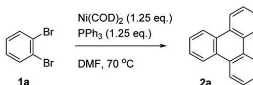
**Scheme 1** Cyclotrimerization of *o*-dibromobenzene using the Yamamoto coupling.<sup>21</sup>
