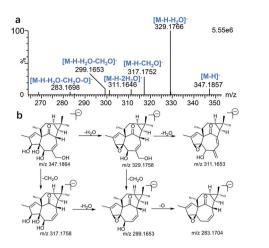
Fig. 3 The Mass spectrum (a) and proposed fragmentation pathways (b) of ingenol.
