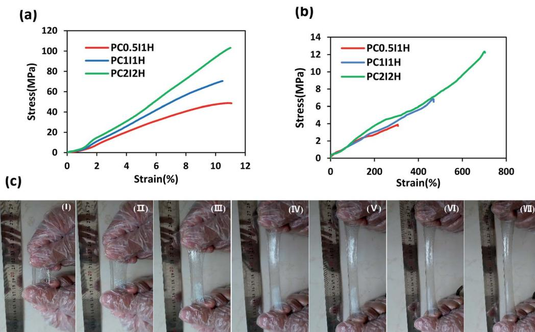
Fig. 6 (a) Tensile stress–strain curves of as-synthesized hydrogel films, (b) tensile stress–strain curves of swollen hydrogel films, (c) photographs of PC<sub>2</sub>I<sub>2</sub>H hydrogel during stretching.
