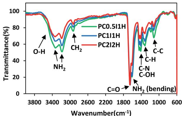
Fig. 2 The ATR-FTIR spectra of freeze-dried hydrogel films.
