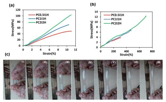
Fig. 6 (a) Tensile stress—strain curves of as-synthesized hydrogel films, (b) tensile stress—strain curves of swollen hydrogel films, (c) photographs of  $PC_2I_2H$  hydrogel during stretching.
