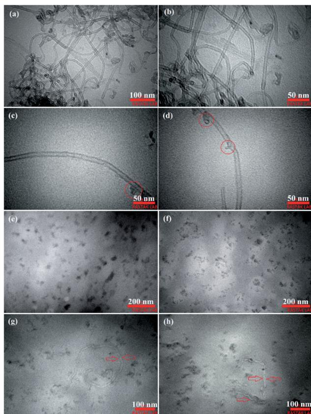
Fig. 5 TEM images of the O-MWCNTs and as-synthesized PC<sub>2</sub>I<sub>2</sub>H film. (a) O-MWCNTs, (b) a high magnification of (a), (c and d) TEM images of a single nanotube with some marked inherent defects, (e) individual O-MWCNT flakes, (f) the flake batches, (g and h) TEM images of incompletely degraded O-MWCNTs among flakes.
