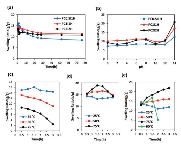
Fig. 8 The swelling ratio curves of different as-synthesized hydrogel films in distilled water at various conditions. (a) At room temperature during 76 h, (b) at different pH values after 76 h, (c-e) at different temperatures during 3 h for PC $_{0.5}I_1H$ , PC $_{11}H$  and PC $_{2}I_2H$  samples, respectively.
