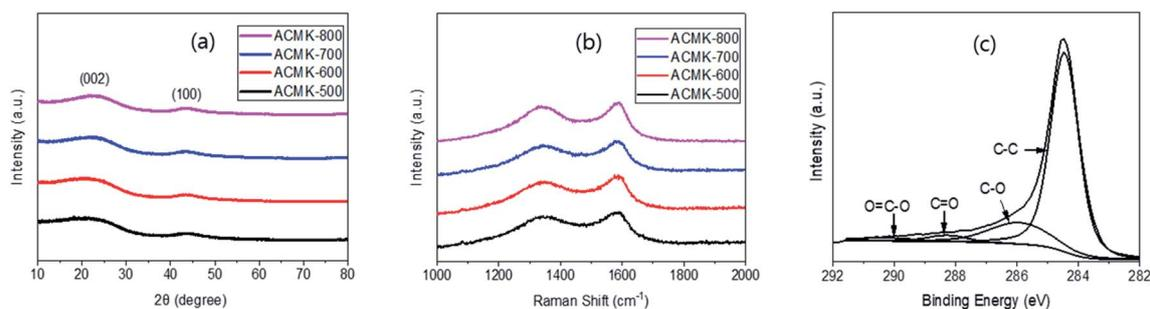
Fig. 3 XRD (a) and Raman (b) of ACMK as well as (c) C<sub>1s</sub> peak of ACMK-500.
