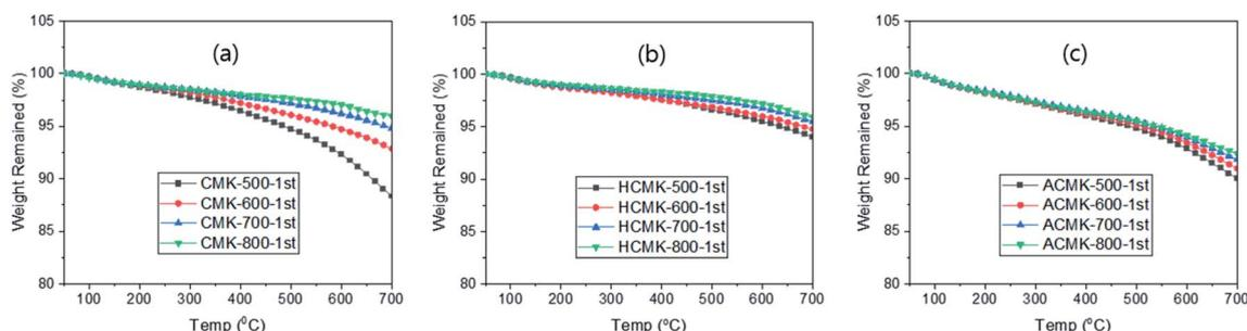
Fig. 1 The 1<sup>st</sup> TGA of CMK (a), HCMK (b) and ACMK (c) under N<sub>2</sub> flow of 20 cc min<sup>-1</sup>.
