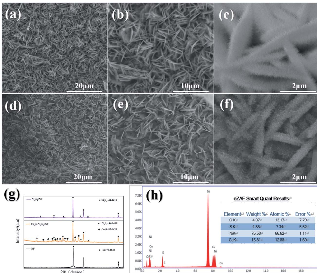
Fig. 2 (a–c) SEM image of NiCu LDH-3, (d–f) SEM image of  $\text{Cu}_2\text{S}/\text{Ni}_3\text{S}_2/\text{NF}$ -3, (g) XRD pattern of  $\text{Ni}_3\text{S}_2/\text{NF}$ ,  $\text{Cu}_2\text{S}/\text{Ni}_3\text{S}_2/\text{NF}$  and NF, (h) EDS image of  $\text{Cu}_2\text{S}/\text{Ni}_3\text{S}_2/\text{NF}$ .
