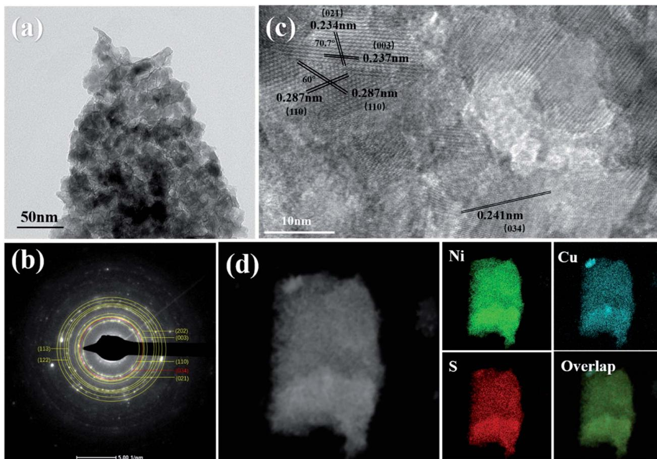
Fig. 4 (a) TEM image of  $\text{Cu}_2\text{S}/\text{Ni}_3\text{S}_2$  layer structure, (b) SAED pattern and (c) HRTEM image of  $\text{Cu}_2\text{S}/\text{Ni}_3\text{S}_2$ , (d) mapping of Ni, Cu, S and overlap images of  $\text{Cu}_2\text{S}/\text{Ni}_3\text{S}_2$  nanosheet.
