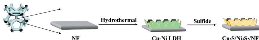
Fig. 1 Schematic diagram of preparation of  $\text{Cu}_2\text{S}/\text{Ni}_3\text{S}_2/\text{NF}$ .
