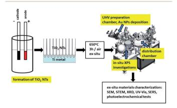
Fig. 1 Schematic diagram of sample preparation and characterization.
