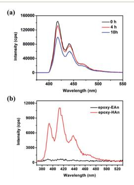
Fig. 3 Fluorescence spectra of (a) epoxy-EAn (0.1%) exposed to 365 nm UV for different time, and (b) leaching solution of epoxy-EAn (0.1%) and epoxy-HAn with consistent molarity of additives (0.56  $\times$  10 $^{-2}$  M).
