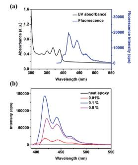
Fig. 1 (a) UV-VIS absorption and fluorescence emission spectrum of epoxy-EAn (EAn concentration of 0.01%). (b) Fluorescence emission spectra of epoxy-EAn with different EAn concentrations.
