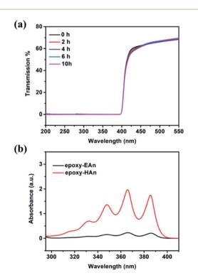
Fig. 6 (a) Transmission curves for epoxy-EAn (0.8%, thickness of 1 mm) exposed to 365 nm UV for different time, and (b) UV absorption of the leaching solution of epoxy-EAn (0.8%) and epoxy-HAn with consistent molarity of additives (4.48  $\times\,10^{-2}$  M).
