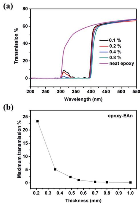
Fig. 5 (a) Transmission curves for the neat epoxy and epoxy-EAn with different EAn concentrations (thickness of 1 mm). (b) Maximum transmission in full test interval vs. the thickness of epoxy-EAn (0.8%).
