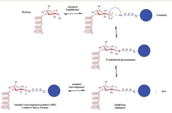
Fig. 3 Schematic representation of the Maillard conjugation reaction between the reducing end of a sugar molecule and a free amine group of a protein, affording a Schiff base and then the Amadori rearrangement product (ARP). This figure has been adapted/reproduced from ref. 68 with permission from the American Chemical Society, 2021.
