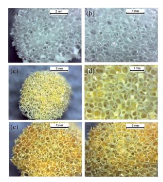
Fig. 9 Digital photographs of coated scaffolds: (a) top surface and (b) cross section of the scaffold coated by PCL (5% w/v), (c) top surface and (d) cross section of the scaffold coated by PCL/zein (2.5%:2.5% w/v) and (e) top surface and (f) cross section of the scaffold coated by zein (5% w/v). This figure has been adapted/reproduced from ref. 160 with permission from Elsevier, 2021.
