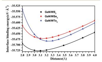
Fig. 2 Plot of interface binding energies as function of interlayer distances for GaN/WS<sub>2</sub>, GaN/WSe<sub>2</sub>, and GaN/WTe<sub>2</sub> heterostructures. 5th order polynomial has been employed for fitting. In order to clarify the equilibrium distances between the GaN layer and WX<sub>2</sub> layer, the values of interface binding energies of both the GaN/WSe<sub>2</sub> and GaN/WTe<sub>2</sub> heterostructures are shifted downwards by 1.80 eV, 5.40 eV, respectively.
