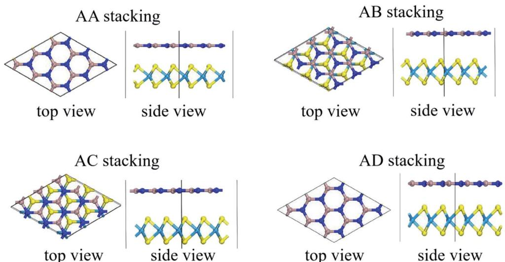
Fig. 1 Relaxed structures of four typical stacking patterns of GaN/WX<sub>2</sub> (X = S, Se, Te) heterostructures. Cyan, yellow, dark blue, and brown spheres indicate W, X, N and Ga atoms, respectively.
