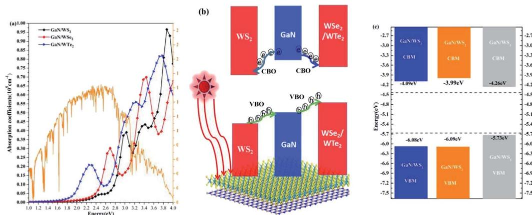
Fig. 5 (a) Absorption spectrum of GaN/WS<sub>2</sub>, GaN/WSe<sub>2</sub>, and GaN/WTe<sub>2</sub> heterostructures. Incident AM 1.5 G solar flux<sup>48</sup> is plotted in orange solid line. (b) Schematic plot of the migration of photogenerated electrons and holes at the GaN/WS<sub>2</sub> interface. (c) Band-edge alignments of GaN/WX<sub>2</sub> heterostructures.
