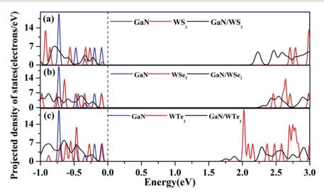
Fig. 4 Projected density of states (PDOS) of (a) GaN/WS<sub>2</sub>, (b) GaN/WSe<sub>2</sub>, and (c) GaN/WTe<sub>2</sub> heterostructures. Fermi level is set to zero as indicated by the black dashed line.
