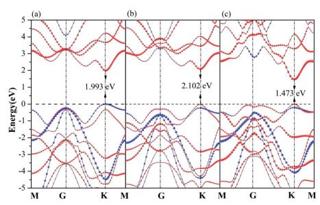
Fig. 3 Projection-resolved band structures of (a)  $GaN/WS_2$ , (b)  $GaN/WS_2$ , and (c)  $GaN/WTe_2$  heterostructures. Blue and red lines indicate contributions from GaN and  $WX_2$  layer, respectively.
