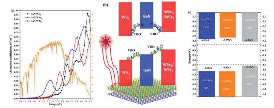
Fig. 5 (a) Absorption spectrum of  $GaN/WS_2$ ,  $GaN/WSe_2$ , and  $GaN/WTe_2$  heterostructures. Incident AM 1.5 G solar flux<sup>48</sup> is plotted in orange solid line. (b) Schematic plot of the migration of photogenerated electrons and holes at the  $GaN/WS_2$  interface. (c) Band-edge alignments of  $GaN/WX_2$  heterostructures.
