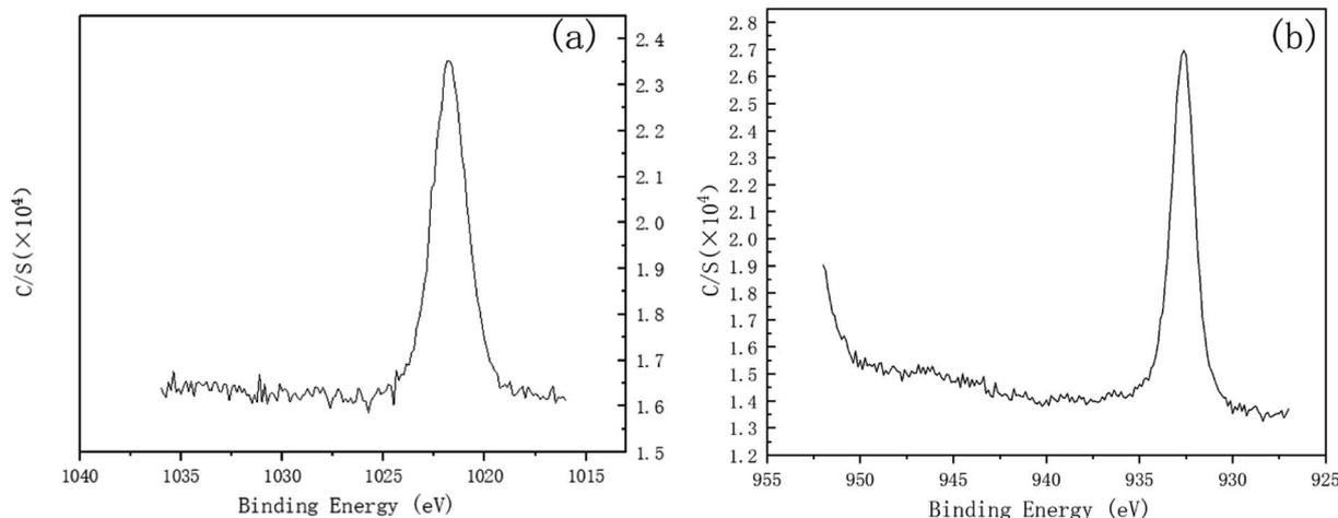
Fig. 8 Zn(2p<sub>3</sub>) and Cu(2p<sub>3</sub>) high-resolution XPS spectra of the specimen after polishing for 120 min at 1.5 V. (a) Zn(2p<sub>3</sub>), (b) Cu(2p<sub>3</sub>).
