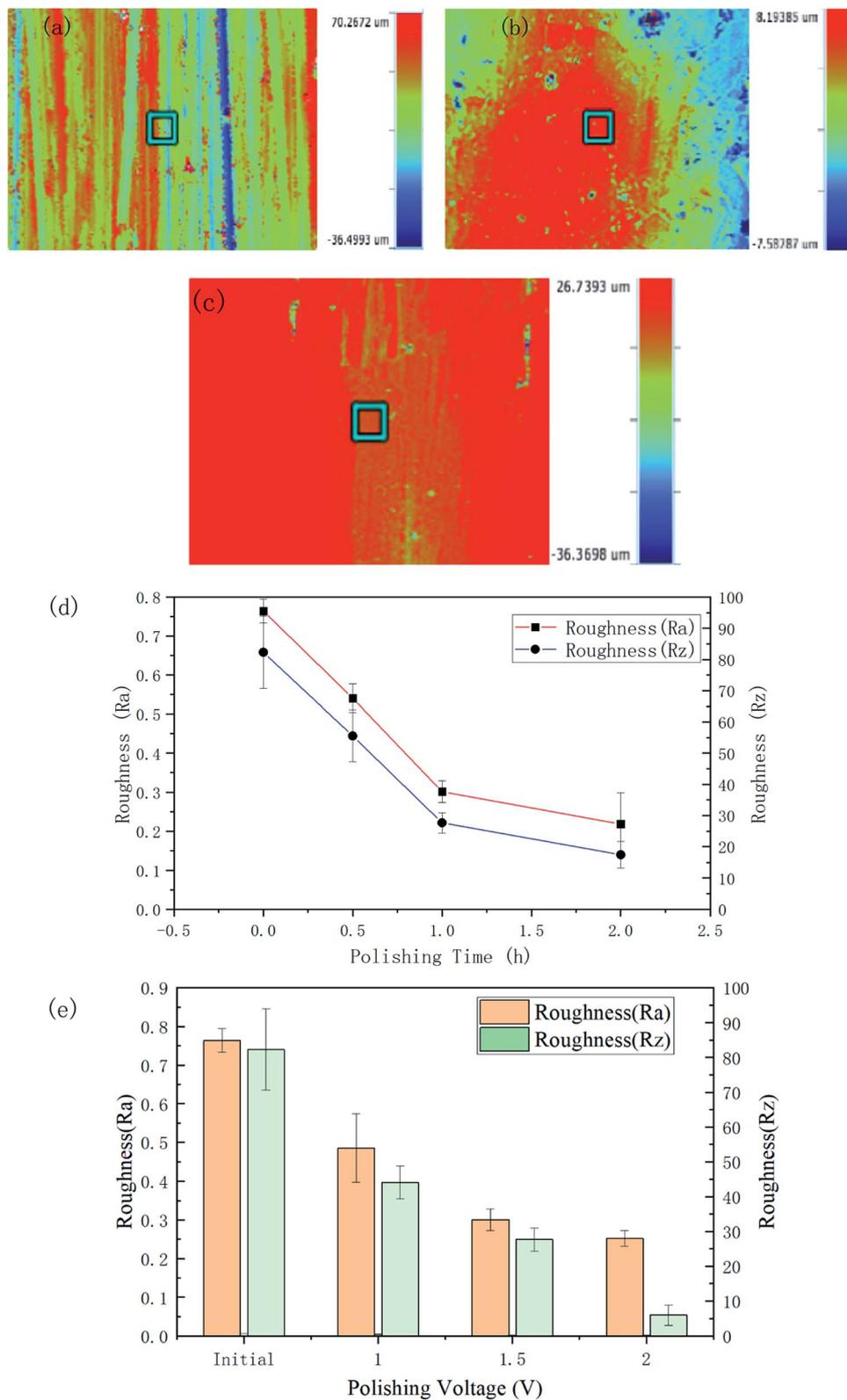
Fig. 6 Surface roughness and 3D contours of the polished specimens at different times/voltages: (a) initial; (b) 1.5 V for 120 min; (c) 2 V for 60 min; (d) and (e) surface roughness comparison in  $R_a$  and  $R_z$ .
