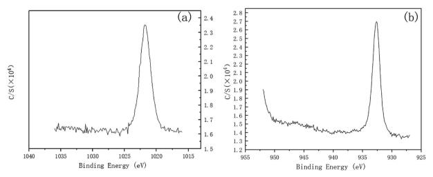
Fig. 8 Zn(2p<sub>x</sub>) and Cu(2p<sub>x</sub>) high-resolution XPS spectra of the specimen after polishing for 120 min at 1.5 V. (a) Zn(2p<sub>x</sub>), (b) Cu(2p<sub>x</sub>).
