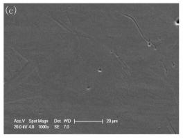
Fig. 5 Surface morphology of the polished specimens at different voltages: (a) 1 V for 60 min; (b) 1.5 V for 60 min; (c) 2 V for 60 min.
