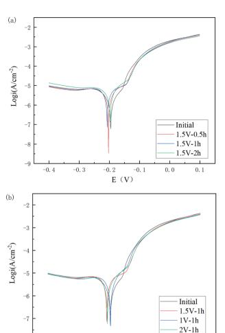
Fig. 11 Tafel plots of Cu 65%–Zn 35% brass specimens with different polishing times (a) and voltages (b).
