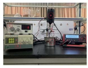
Fig. 2 DECP polishing devices: (a) digital display electric stirrer; (b) DC power supply; (c) a 304 stainless steel container; (d) digital display multimeter.
