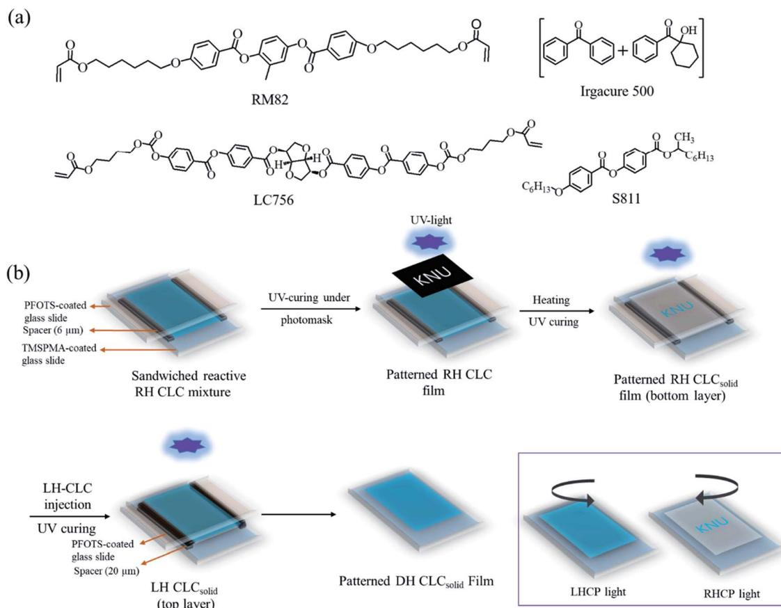
**Fig. 1** (a) Chemical structures of diacrylate mesogens (RM82), reactive right-handed (RH) chiral dopant (LC756), nonreactive left-handed (LH) chiral dopant (S-811), and photo-initiator (Irgacure 500) used in the preparation of the reactive cholesteric liquid crystal (CLC) mixtures. (b) Schematic representation of the preparation procedure of the patterned dual-handed (DH) bilayer solid-state CLC ( $\text{CLC}_{\text{solid}}$ ) film.
