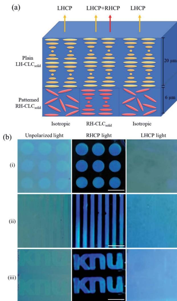
Fig. 3 (a) Schematic representation of the internal structure and handedness of the fabricated double-handed (DH)-solid-state cholesteric liquid crystal (CLC<sub>solid</sub>) film. (b) Photographic images of the (i) dots, (ii) lines, and (iii) "KNU" letter patterns of the DH-CLC<sub>solid</sub> films under unpolarized, right-handed circularly polarized (RHCP), and left-handed circularly polarized (LHCP) lights. The scale bars are 4 mm.
