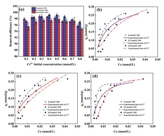
Fig. 9 Influence of the MO and  $Cr(v_1)$  concentration on the adsorption of  $Cr(v_1)$  onto Fe@LS-BC (a), Langmuir (b), Freundlich (c), Langmuir-Freundlich (d) isotherms (pH 2; adsorbent dose 4 g L<sup>-1</sup>; temperature 298 K; contact duration 90 min;  $Cr(v_1)$  concentration between 0.1–0.8 mmol L<sup>-1</sup>; MO concentrations of 0, 0.2, and 0.8 mmol L<sup>-1</sup>, accordingly).
