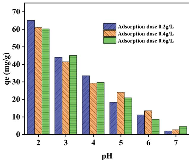
Fig. 7 Impact of pH on the adsorption of Cr(VI) on Fe@LS-BC (Cr(VI) concentration 50 mg L<sup>-1</sup>; pH 2–7; constant duration 360 min; temperature 298 K; adsorbent dose 0.2, 0.4, and 0.6 g L<sup>-1</sup>, respectively).
