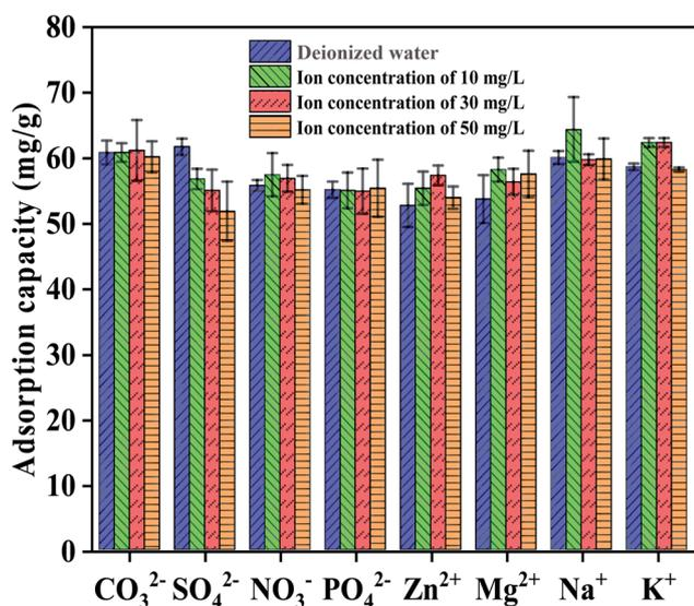
Fig. 8 Influence of ionic strength on Cr(VI) removal (pH 2; adsorbent dose 0.2 g L<sup>-1</sup>; temperature 298 K; contact duration 360 min; Cr(VI) concentration 50 mg L<sup>-1</sup>; anion concentrations of 10, 30, and 50 mg L<sup>-1</sup>, respectively).
