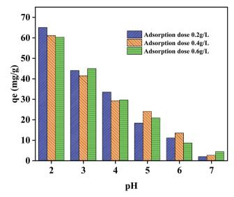
Fig. 7 Impact of pH on the adsorption of Cr(vi) on Fe@LS-BC (Cr(vi) concentration 50 mg L $^{-1}$ ; pH 2-7; constant duration 360 min; temperature 298 K; adsorbent dose 0.2, 0.4, and 0.6 g L $^{-1}$ , respectively).
