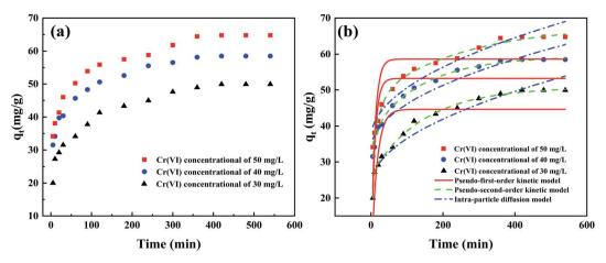
Fig. 6 Influence of time on  $Cr(v_i)$  adsorption by Fe@LS-BC (a); pseudo-first-order, pseudo-second-order, and intraparticle diffusion adsorption kinetics for  $Cr(v_i)$  adsorption on Fe@LS-BC (b) (contact duration 5–540 min; adsorbent dose 0.4 g  $L^{-1}$ ; pH 2; primary concentration of  $Cr(v_i)$  was 30, 40, and 50 mg  $L^{-1}$ , respectively; temperature 298 K).
