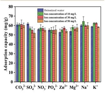
Fig. 8 Influence of ionic strength on  $Cr(v_1)$  removal (pH 2; adsorbent dose 0.2 g  $L^{-1}$ ; temperature 298 K; contact duration 360 min;  $Cr(v_1)$  concentration 50 mg  $L^{-1}$ ; anion concentrations of 10, 30, and 50 mg  $L^{-1}$ , respectively).
