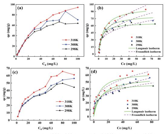
Fig. 5 Influence of the primary concentration of  $Cr(v_1)$  on  $Cr(v_1)$  adsorption by Fe@LS-BC (a); isotherm models of  $Cr(v_1)$  through Fe@LS-BC (b); influence of the primary concentration of  $Cr(v_1)$  on  $Cr(v_1)$  adsorption by LS-BC (c); isotherm models of  $Cr(v_1)$  through LS-BC (d) (primary concentration of  $Cr(v_1)$  ranged from 2–100 mg  $L^{-1}$ ; pH 2, constant duration 360 min; temperature 298, 308, and 319 K, respectively; adsorbent dose 0.4 g  $L^{-1}$ ).
