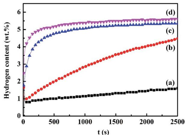
Fig. 5 Absorption kinetics curves of ball-milled samples at different temperatures under 3.0 MPa H<sub>2</sub>:MgH<sub>2</sub> at 473 K (a) and 523 K (b) and Ce<sub>0.8</sub>Fe<sub>0.1</sub>Zr<sub>0.1</sub>O<sub>2</sub>-catalyzed MgH<sub>2</sub> at 473 K (c) and 523 K (d).
