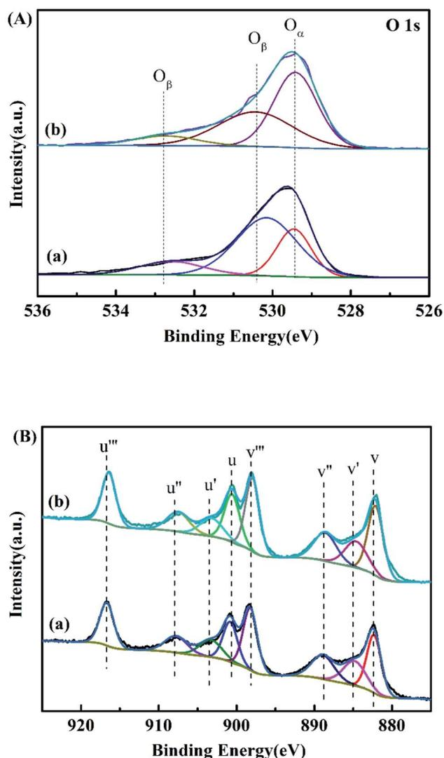
Fig. 8 (A) O 1s XPS spectra of (a) CeO<sub>2</sub> and (b) Ce<sub>0.8</sub>Fe<sub>0.1</sub>Zr<sub>0.1</sub>O<sub>2</sub>; (B) Ce 3d XPS spectra of (a) CeO<sub>2</sub> and (b) Ce<sub>0.8</sub>Fe<sub>0.1</sub>Zr<sub>0.1</sub>O<sub>2</sub>.
