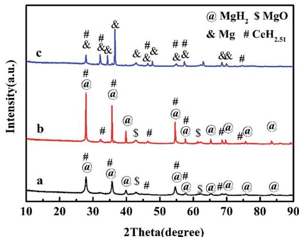
Fig. 7 XRD patterns of  $\text{Ce}_{0.8}\text{Fe}_{0.1}\text{Zr}_{0.1}\text{O}_2$ -catalyzed  $\text{MgH}_2$  at different stages: (a) after ball-milling, (b) hydrogenation at 3.0 MPa and (c) dehydrogenation at 623 K.
