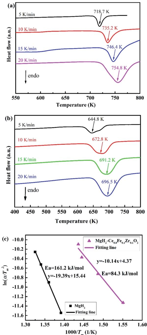
Fig. 4 DSC curves of MgH<sub>2</sub> (a) and Ce<sub>0.8</sub>Fe<sub>0.1</sub>Zr<sub>0.1</sub>O<sub>2</sub>-catalyzed MgH<sub>2</sub> (b) at different heating rates; (c) Kissinger's plots for milled MgH<sub>2</sub> and MgH<sub>2</sub>-Ce<sub>0.8</sub>Fe<sub>0.1</sub>Zr<sub>0.1</sub>O<sub>2</sub> composite.
