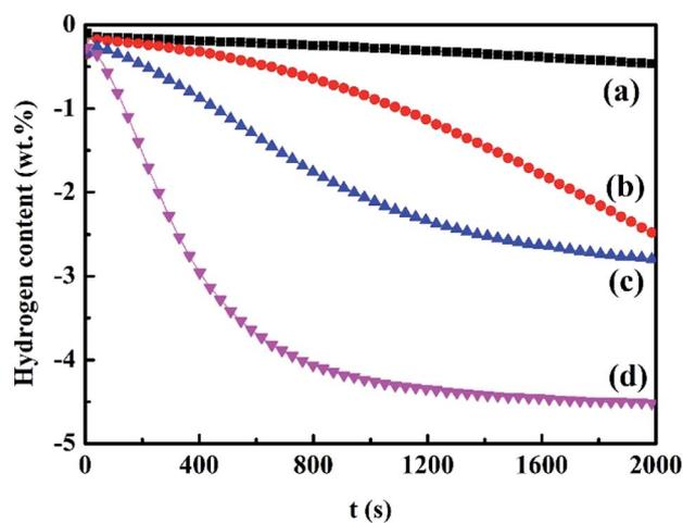
Fig. 3 Desorption kinetics curves of ball-milled  $\text{MgH}_2$  at 598 K (a) and 623 K (b) and  $\text{Ce}_{0.8}\text{Fe}_{0.1}\text{Zr}_{0.1}\text{O}_2$  catalyzed  $\text{MgH}_2$  at 598 K (c) and 623 K (d).
