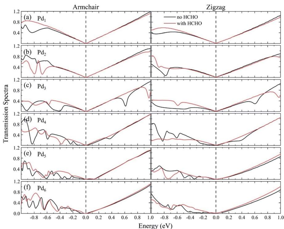
Fig. 9 Transmission spectra for the  $\text{Pd}_n$ /graphene ( $n = 1-6$ ) sensors without and with HCHO adsorption at zero bias are shown in (a-f). The dashed lines, which are set to be zero on the energy scale, indicate the Fermi level.
