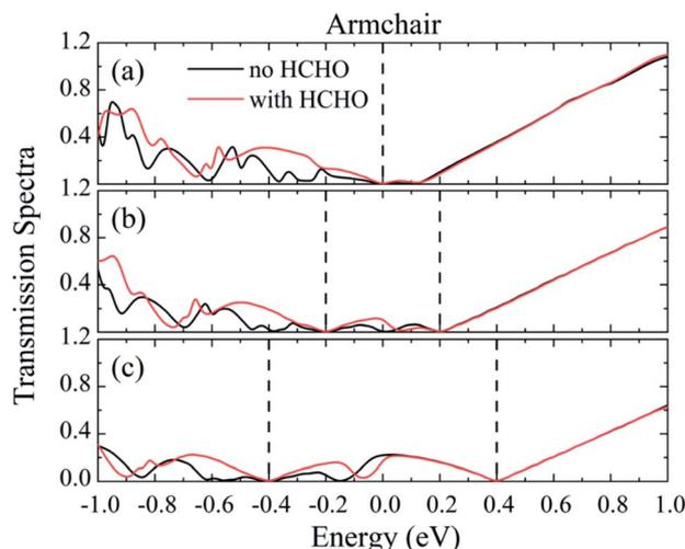
Fig. 10 The transmission spectra of HCHO nano-sensor constructed from Pd<sub>5</sub>/graphene along the armchair-direction under (a–c) 0, 0.4 and 0.8 V bias. The dashed lines represent the bias windows.
