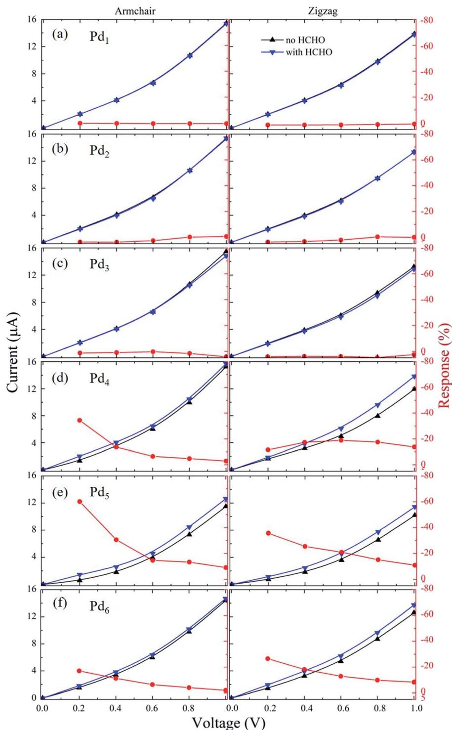
Fig. 8 The current–voltage curves and responses of the armchair- and zigzag-orientated nano-sensor devices constructed from Pd<sub>n</sub>/graphene ( $n = 1-6$ ) under the bias voltage from 0 to 1.0 V are presented in (a–f).
