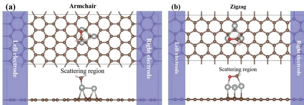
Fig. 7 Two-probe nano-sensor device models, using HCHO adsorption on Pd<sub>3</sub>/graphene as the example. The semi-infinite left and right graphene electrodes (shaded zones) are in contact with the scattering region. Both the top and side views of the devices along the armchair (a) and zigzag (b) directions are shown. The C, Pd, O and H atoms are shown in brown, silver, red and white balls, respectively.
