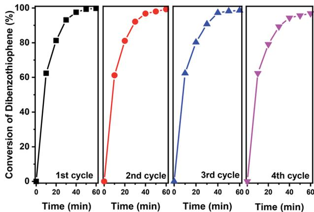
Fig. 8 Photocatalytic degradation of DBT in successive cycles by 40%  $V_2O_5/Fe-Al-SBA-15$ . (Reaction conditions:  $V_{model\ oil} = 50\ ml$ ,  $m_{catalyst} = 50\ mg$ ,  $V_{H_2O_2} = 1.0\ ml$ , at a reaction temperature of  $70\ ^\circ C$ ).
