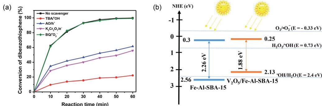
Fig. 9 (a) The active-species-trapping experiments for conversion of DBT over 40%  $V_2O_5/Fe-Al-SBA-15$  photocatalyst. (b) The schematic of the separation and transfer of photogenerated charges over  $V_2O_5/Fe-Al-SBA-15$ .
