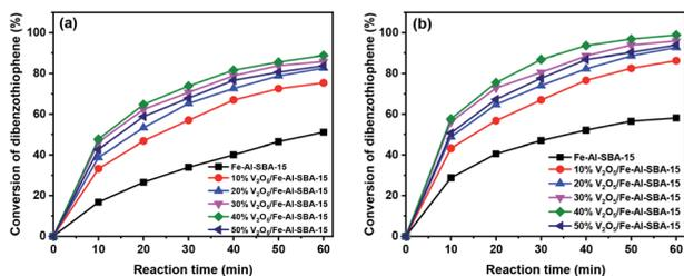
Fig. 7 Photodegradation of DBT (500 ppm of DBT in 100 ml *n*-octane solution) with different photocatalysts (50 mg of photocatalyst and 1 ml of  $H_2O_2$ ) under sunlight irradiation at reaction temperatures of (a) 40 °C and (b) 60 °C.
