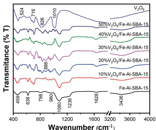
Fig. 2 FT-IR spectra of  $V_2O_5$  and  $V_2O_5/Fe-Al-SBA-15$  samples.
