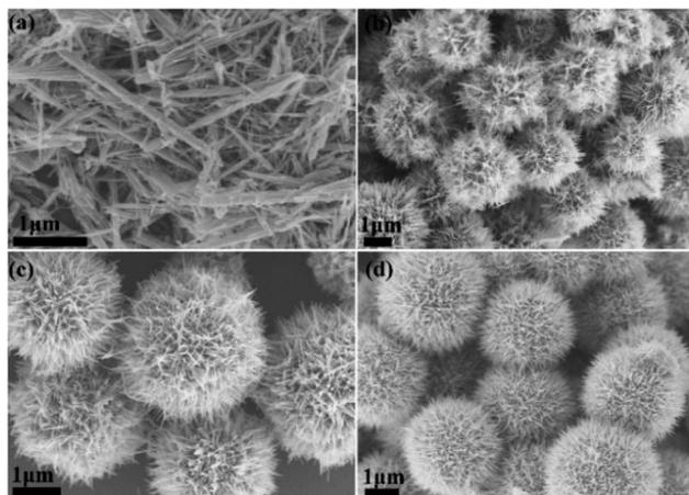
Fig. 4 FESEM and TEM images of the  $\gamma$ -MnO<sub>2</sub> mesocrystals obtained after 12 h with a constant Mn(II) concentration of 0.1 mol L<sup>-1</sup> and various collagen concentrations: (a) 0 wt%; (b) 0.02 wt%; (c) 0.05 wt%; (d) 0.2 wt%.
