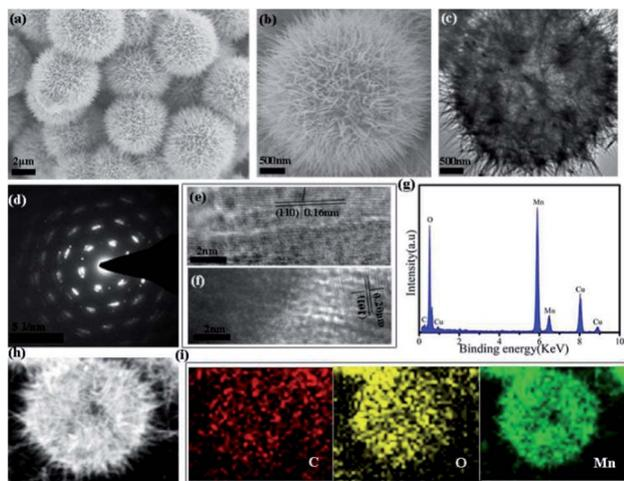
Fig. 1 Characterization of the morphology of the  $\gamma$ -MnO<sub>2</sub> mesocrystals obtained after 12 h *via* collagen-templated biomineralization ([collagen] = 0.1 wt%, [Mn(II)] = 0.1 mol L<sup>-1</sup>): (a and b) FESEM images; (c) TEM image; (d) the SAED pattern; (e and f) HRTEM images; (g) EDX spectrum; (h) HAADF-STEM images; (i) EDS mapping images of C, O, and Mn for the  $\gamma$ -MnO<sub>2</sub> in (h).
