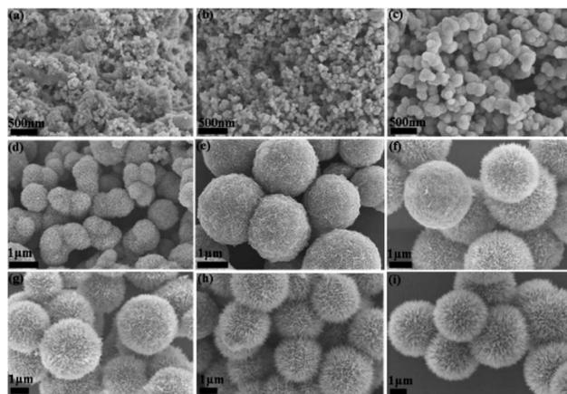
Fig. 2 FESEM images of the  $\gamma$ -MnO<sub>2</sub> mesocrystals obtained *via* collagen-templated biomineralization ([collagen] = 0.1 wt%, [Mn(II)] = 0.1 mol L<sup>-1</sup>) by different incubation time: (a) 10 min; (b) 15 min; (c) 30 min; (d) 45 min; (e) 60 min; (f) 90 min; (g) 120 min; (h) 2.5 h; (i) 4 h.
