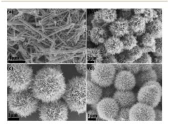
Fig. 4 FESEM and TEM images of the  $\gamma$ -MnO<sub>2</sub> mesocrystals obtained after 12 h with a constant Mn(II) concentration of 0.1 mol L<sup>-1</sup> and various collagen concentrations: (a) 0 wt%; (b) 0.02 wt%; (c) 0.05 wt%; (d) 0.2 wt%.
