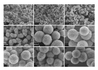
Fig. 2 FESEM images of the  $\gamma$ -MnO<sub>2</sub> mesocrystals obtained *via* collagen-templated biomineralization ([collagen] = 0.1 wt%, [Mn( $\parallel$ )] = 0.1 mol L<sup>-1</sup>) by different incubation time: (a) 10 min; (b) 15 min; (c) 30 min; (d) 45 min; (e) 60 min; (f) 90 min; (g) 120 min; (h) 2.5 h; (i) 4 h.
