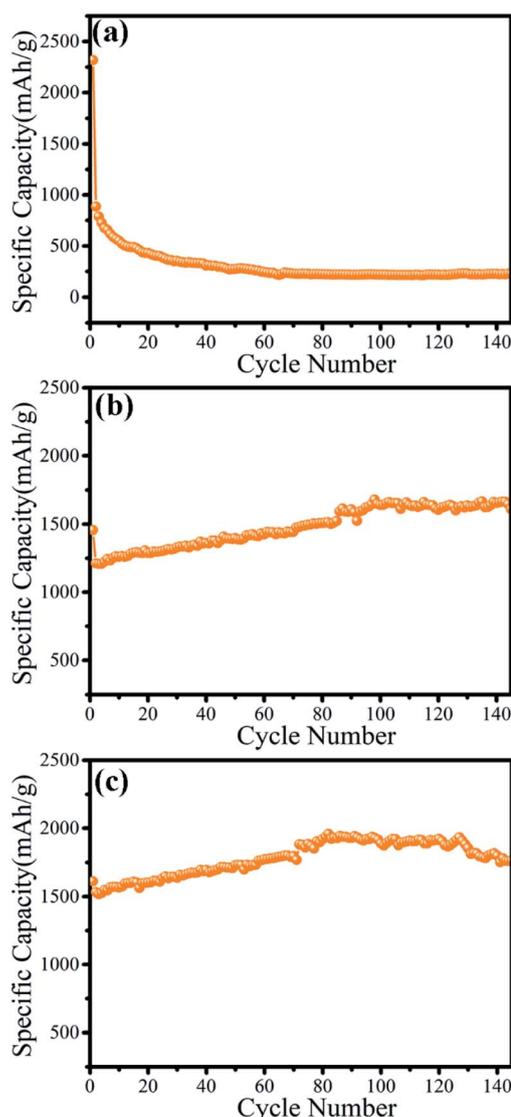
Fig. 5 The cycling performance of  $\gamma$ -MnO<sub>2</sub> mesocrystals prepared by different concentrations of collagen: (a) 0; (b) 0.05 wt%; (c) 0.1 wt%.
