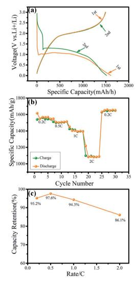
Fig. 6 Electrochemical properties of the  $\gamma$ -MnO<sub>2</sub> electrodes. (a) The charge/discharge profiles of  $\gamma$ -MnO<sub>2</sub> electrode at 0.2C between 0.01 to 3.0 V; (b) rate capacities of  $\gamma$ -MnO<sub>2</sub> at different current densities from 0.2C to 2.0C; (c) capacity retention of  $\gamma$ -MnO<sub>2</sub> at different rates.
