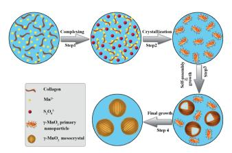
Scheme 1 Schematic illustration of the essential role of collagen in the modulation of hollow dandelion-like microspheres of  $\gamma$ -MnO<sub>2</sub> mesocrystals.
