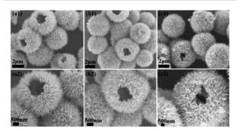
Fig. 3 Observation of some incomplete microspheres in the FESEM images of the  $\gamma$ -MnO<sub>2</sub> mesocrystals obtained after 2 h *via* collagentemplated biomineralization ([collagen] = 0.1 wt%, Mn(II) = 0.1 mol L<sup>-1</sup>).
