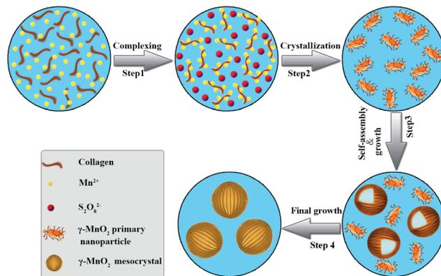
Scheme 1 Schematic illustration of the essential role of collagen in the modulation of hollow dandelion-like microspheres of  $\gamma$ -MnO<sub>2</sub> mesocrystals.
