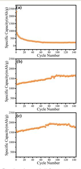
Fig. 5 The cycling performance of  $\gamma$ -MnO<sub>2</sub> mesocrystals prepared by different concentrations of collagen: (a) 0; (b) 0.05 wt%; (c) 0.1 wt%.
