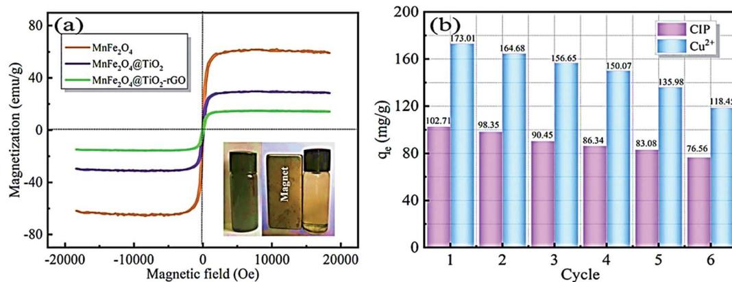
Fig. 15 (a) Magnetic properties of the prepared composite, (b) reusability of the prepared composite for the adsorption of CIP and Cu<sup>2+</sup>, adapted with permission from ref. 122, copyright, Elsevier, 2021.
