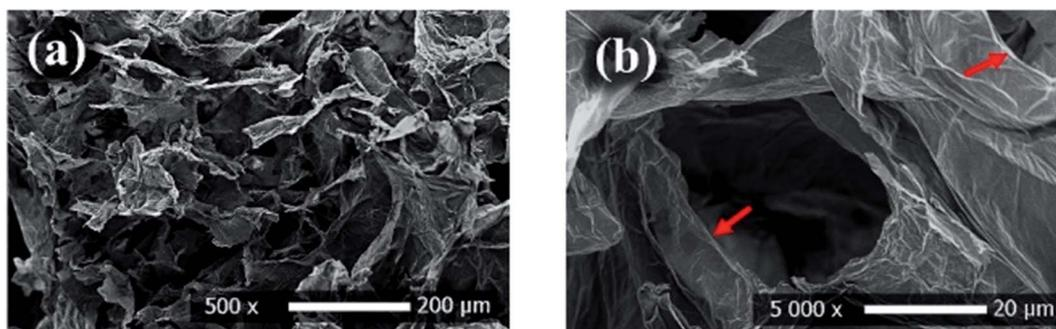
Fig. 13 SEM images (a and b) of rGO showing its unique layered structure, adapted with permission from ref. <sup>117</sup>, copyright, American Chemical Society, 2021.
