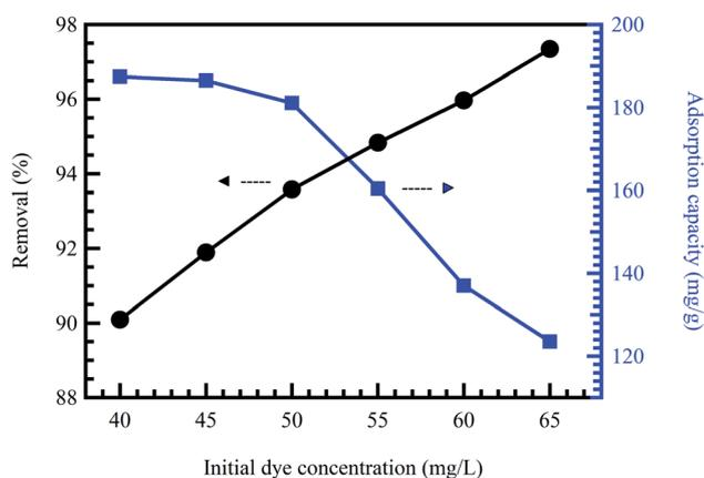
Fig. 5 Effect of initial MB concentration onto ZnCl<sub>2</sub> corn husk AC adsorbent at pH = 4, and adsorbent dose = 0.3 g L<sup>-1</sup>, reproduced with permission from ref. 55, copyright, Hindawi, 2013.
