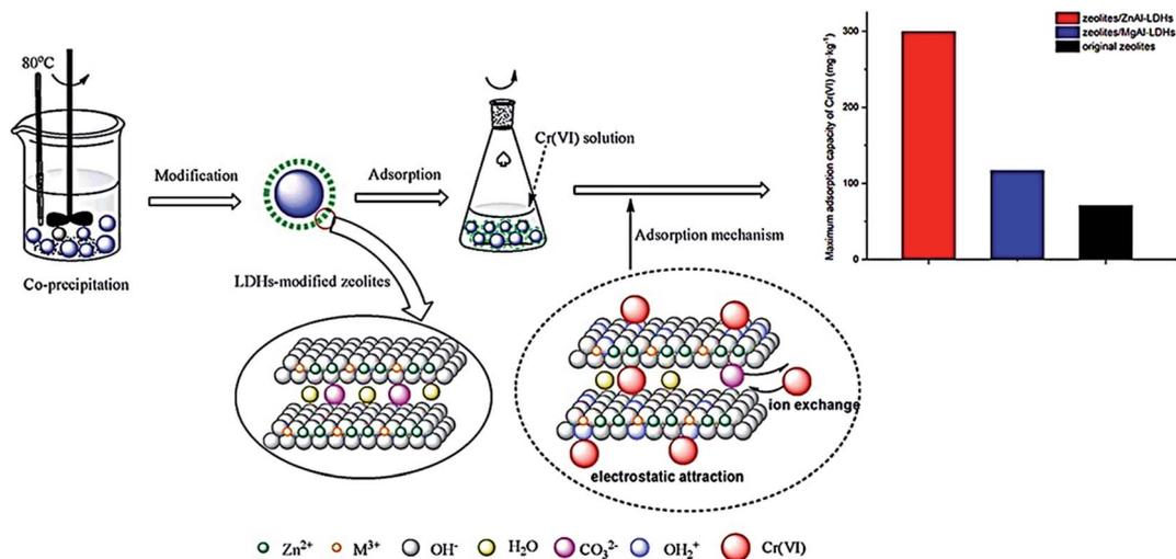
Fig. 17 Removal difference of Cr<sup>6+</sup> by modified zeolites coated with MgAl and ZnAl-layered double hydroxides, adapted with permission from ref. 170, copyright, Elsevier, 2021.
