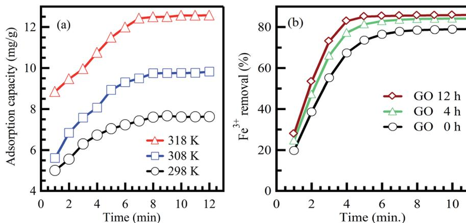
Fig. 4 Effect of contact time on the adsorption of (a) bromothymol blue dye on polyvinyl alcohol adsorbent, adapted with permission from ref. 49, copyright, Elsevier, 2016, and (b) Fe<sup>3+</sup> on graphene oxide aerogel adsorbent, adapted with permission from ref. 50, copyright, Elsevier, 2019.
