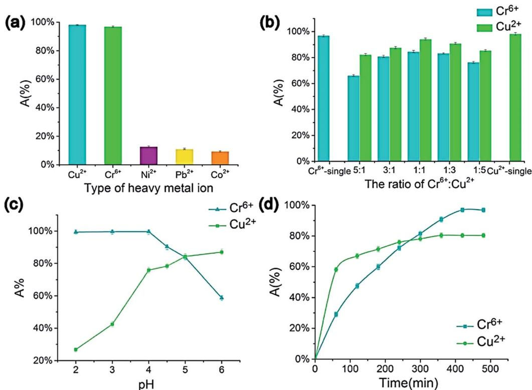
Fig. 11 Impacts of metal ions' type (a) Cr<sup>6+</sup> to Cu<sup>2+</sup> ratio, (b) pH, (c) adsorption time, and (d) on the metal ions' adsorption efficiency (composite tablet adsorbed with 10 mg L<sup>-1</sup> concentration under 40 °C temperature for 600 min in 4.5 pH, 5 mL of metal ion aqueous solution (1 mg L<sup>-1</sup>), 130 rpm), adapted with permission from ref. 104, copyright, Elsevier, 2021.
