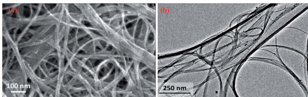
**Fig. 8** SEM (a) and TEM (b) images showing the morphology of SWCNTs, adapted with permission from ref. 91, copyright, Elsevier, 2016.**Table 4** Recent reports on the various preparation routes of CNTs-based and their properties
