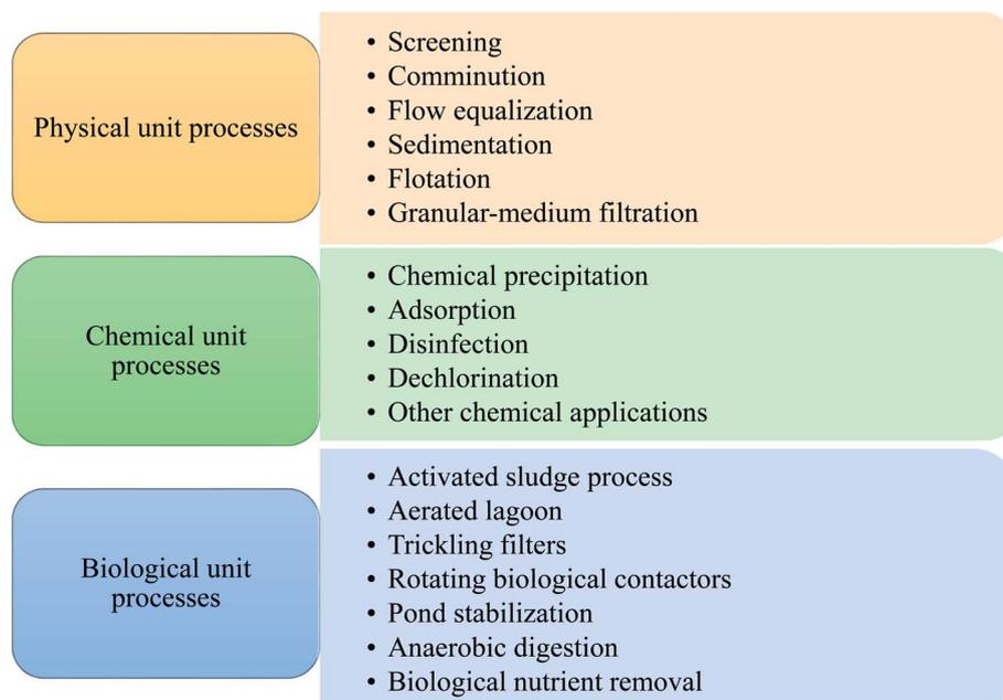
**Fig. 1** Wastewater treatment unit operations and processes.
