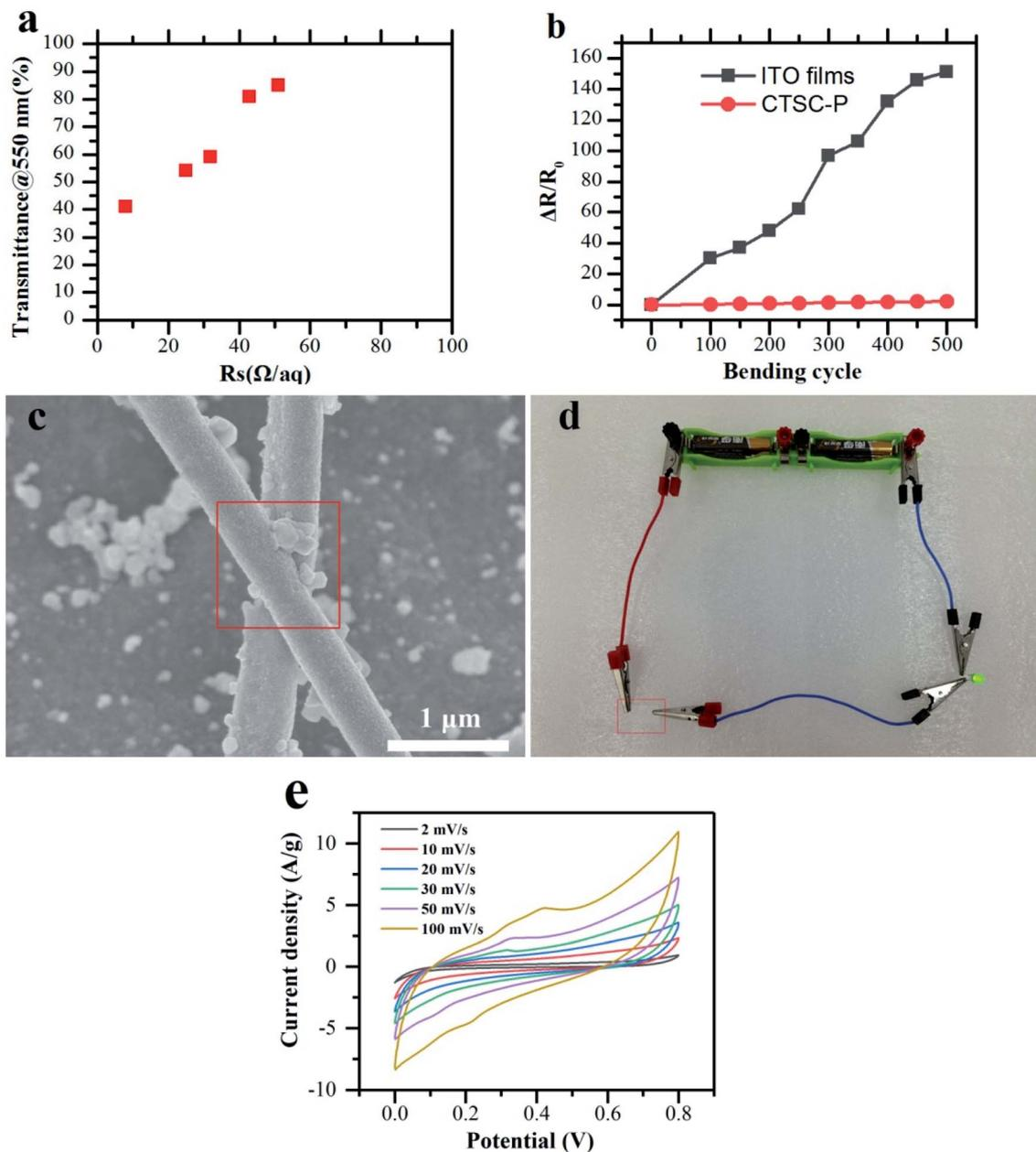
Fig. 8 Electrical conductivity of transparent, flexible, superhydrophobic cellulose films. (a)  $R_s - T$  performance of CTSC-P. (b) Percentage sheet resistance change after 500 bending cycles. (c) SEM of Ag wire. The electroless desposition covers the whole junction, explaining the high performance of electricity. (d) Photo of CTSC-P with a power supply (2.3 V) lighting a green LED device. (e) CV curves at different scan rates of CTSC-P.
