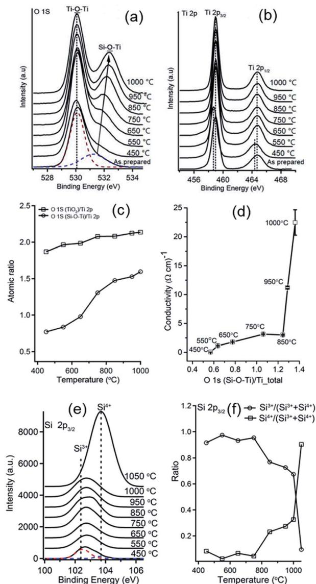
**Fig. 5** XPS analysis for Si–Ti LO films after calcination at specified temperatures under Ar measured under vacuum at RT. (a) O1s XPS spectra (b) Ti2p XPS spectra (c) O1s(TiO<sub>2</sub>)/Ti2p atomic ratios of indicated species vs. temperatures. (d) Film conductivity vs. O1s{Si–O–Ti}/Ti2p ratios. (e) Si2p XPS spectra (f) relative contribution of Si<sup>3+</sup> and Si<sup>4+</sup> species. Si–Ti LO films ( $m = 1$ ,  $n = 5$ ,  $L = 120$ , DM-APTMS).
