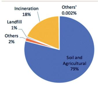
Fig. 5 Sewage sludge disposal techniques in the UK (2010).79
