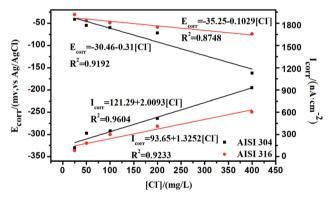
Fig. 8 Potentiodynamic polarization test for AISI 304 and AISI 316.
