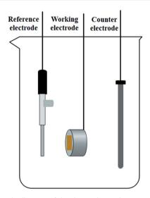
Fig. 1 Schematic diagram of the three-electrode test cell.
