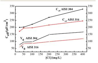
Fig. 4 Admittance ( $Y_0$ ) and calculated effective capacitance ( $C_{\rm eff}$ ) of AISI 304 and AISI 316 at different chloride concentration.
