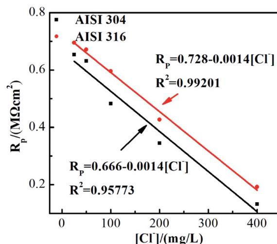
Fig. 6  $R_p$  of EIS experimental data for AISI 304 and AISI 316 at different chloride concentration.
