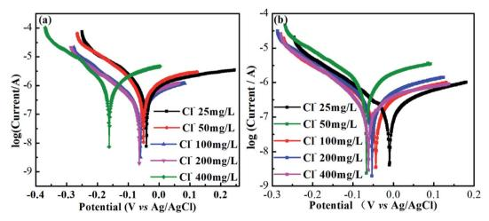
Fig. 7 Polarization curves for AISI 304 (a) and AISI 316 (b) at different chloride concentration.
