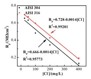
Fig. 6  $\,$   $R_{\rm P}$  of EIS experimental data for AISI 304 and AISI 316 at different chloride concentration.
