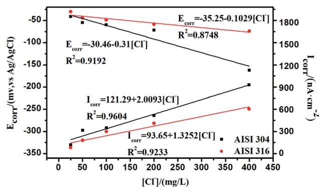
Fig. 8 Potentiodynamic polarization test for AISI 304 and AISI 316.
