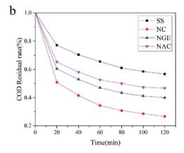
Fig. 14 TOC and COD of PNP degradation. Conditions: pH = 5, voltage 5 V, 0.05 M Na<sub>2</sub>SO<sub>4</sub> and a constant temperature of 20 °C.
