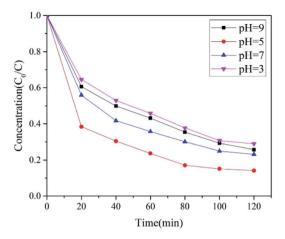
Fig. 10 Effect of pH on PNP degradation. Conditions: pH = 5, voltage 5 V, 0.05 M Na<sub>2</sub>SO<sub>4</sub> and a constant temperature of 20 °C.
