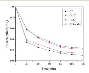
Fig. 13 The effect of background ions on PNP degradation. Conditions: pH = 5, voltage 5 V, 0.05 M  $Na_2SO_4$  and a constant temperature of 20  $^{\circ}C$ .
