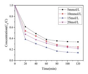
Fig. 12 The effect of PMS concentration on PNP degradation. Conditions: pH = 5, voltage 5 V, 0.05 M  $Na_2SO_4$  and a constant temperature of 20 °C.
