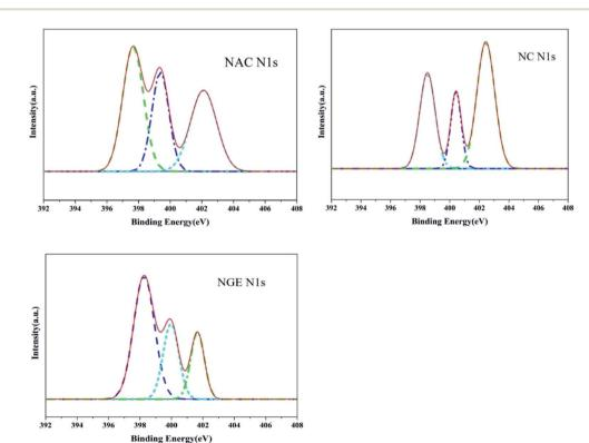
Fig. 3 XPS high-resolution N1s spectra of NGE, NAC and NC.
