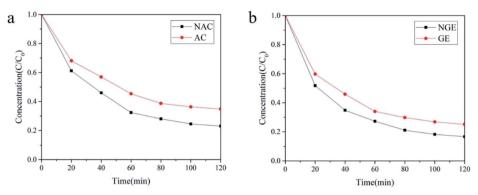
Fig. 8 (a) The effect of NAC and AC on PNP degradation; (b) The effect of NGE and GE on PNP degradation.
