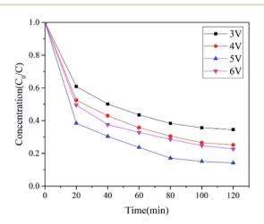
Fig. 11 The effect of voltage on PNP degradation. Conditions: pH = 5, voltage 5 V, 0.05 M Na<sub>2</sub>SO<sub>4</sub> and a constant temperature of 20 °C.
