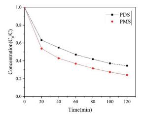
Fig. 7 The effect of oxidant on PNP degradation.
