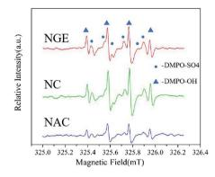
Fig. 16 ESR spectrum in the E-NC-PMS, E-NAC-PMS and E-NGE-PMS systems. Conditions: pH = 5, voltage 5 V, 0.05 M  $Na_2SO_4$  and a constant temperature of 20 °C.
