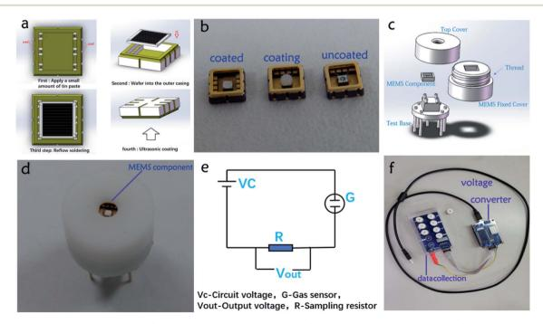
Fig. 1 (a) Processing of MEMS component; (b) coating materials on the MEMS; (c) the test base of MEMS gas sensor; (d) the entity of test base; (e) measuring circuit of MEMS gas sensor made by the author; (f) the test system of MEMS gas sensor made by our lab.
