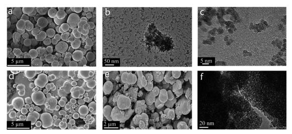
Fig. 4 (a) is the FESEM of  $SnO_2$  get in 125 °C for 3 h, (b) is get from (a) that after ultrasonic treatment for five minutes, (c) is part of (b and d) is the FESEM of  $SnO_2$  get in 135 °C for 3 h, (e) is get from d that after ultrasonic treatment for five minutes, (f) is the TEM of (e).
