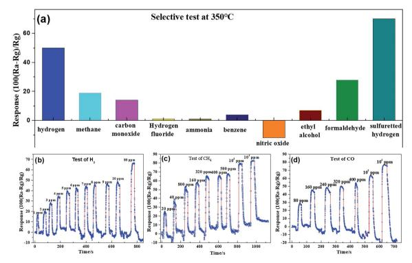
Fig. 6 Gas sensitivity test of combustible gas at 350 °C. (a) Is a selective test of the material for ten common gases. (b) Is the response of the material to  $H_2$  (1–80 ppm). (c) Is the response of the material to methane (20–10 000 ppm). (d) Is the response to carbon monoxide (80–10 000 ppm).
