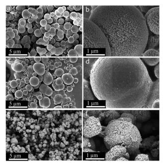
Fig. 3 FESEM image of  $SnO_2$  to different reaction condition. (a and b) is the  $SnO_2$  that get in 125 °C for 3 h; (c and d) is the  $SnO_2$  that get in 135 °C for 3 h; (e and f) is the  $SnO_2$  that get in 180 °C for 3 h.
