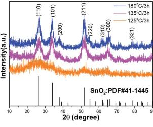
Fig. 2 X-ray diffraction patterns of  $SnO_2$  to different reaction condition.
