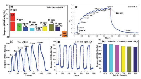
Fig. 5 Sensitivity test of material to hydrogen sulfide at 50 °C. (a) is the test of selectivity. (b) is the test of concentration gradient. (c) is the test of different concentration to  $H_2S$ . (d) is the test of 1 ppm  $H_2S$ . (e) is the effect of humidity on performance.
