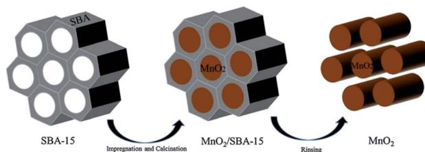
Fig. 4 Schematic representation of the preparation of  $MnO_2$  by SBA-15 template. Reproduced by Zhang *et al.*<sup>80</sup> with permission from Elsevier.
