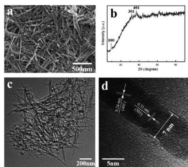
Fig. 3 (a) SEM image, (b) XRD pattern, (c) and (d) TEM images of  $MnO_2$  nanowire prepared by sol-gel approach. Reproduced by Tang *et al.*<sup>55</sup> with permission from Elsevier.
