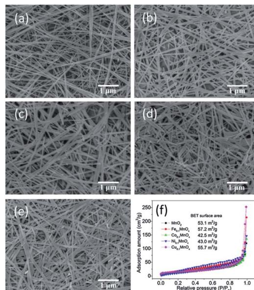
Fig. 9 SEM images of (a) MnO<sub>2</sub>, (b) Fe<sub>0.1</sub>MnO<sub>x</sub>, (c) Co<sub>0.1</sub>MnO<sub>x</sub>, (d) Ni<sub>0.1</sub>MnO<sub>x</sub>, and (e) Cu<sub>0.1</sub>MnO<sub>x</sub> nanowires and (f) N<sub>2</sub> adsorption-desorption isotherms. Reproduced by Gao *et al.*<sup>61</sup> with permission from Elsevier.
