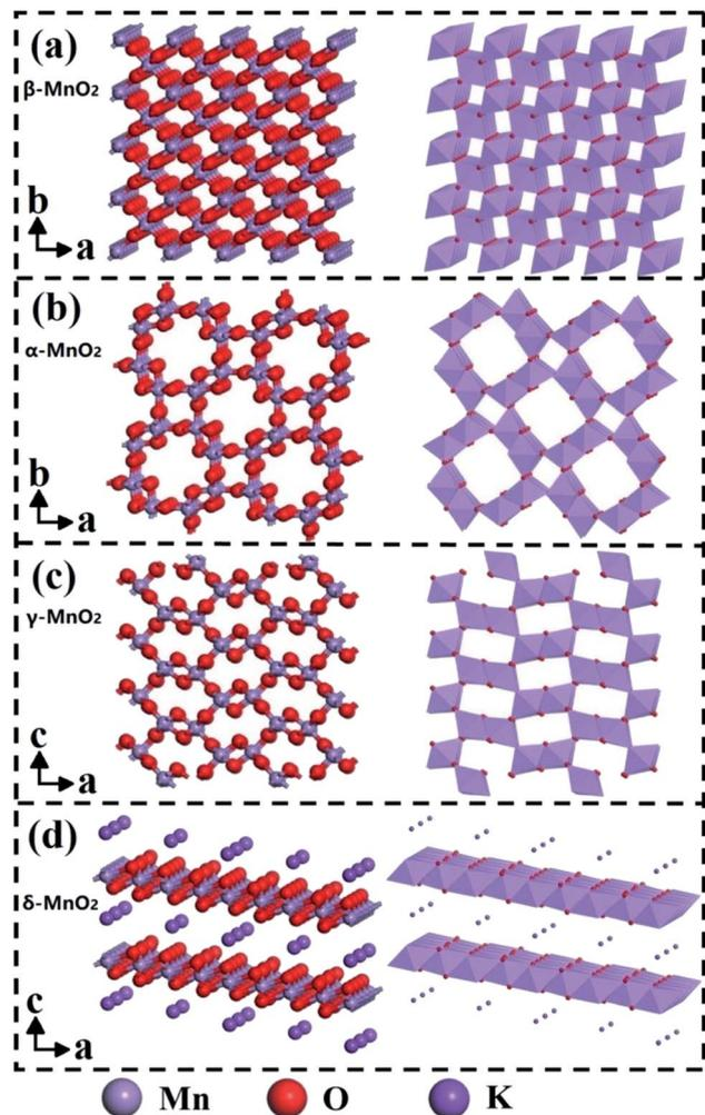
Fig. 5 Ball-stick and polyhedron representations of (a)  $\beta$ -, (b)  $\alpha$ -, (c)  $\gamma$ - and (d)  $\delta$ - $\text{MnO}_2$ . Reproduced by Li *et al.*<sup>91</sup> with permission from Elsevier.
