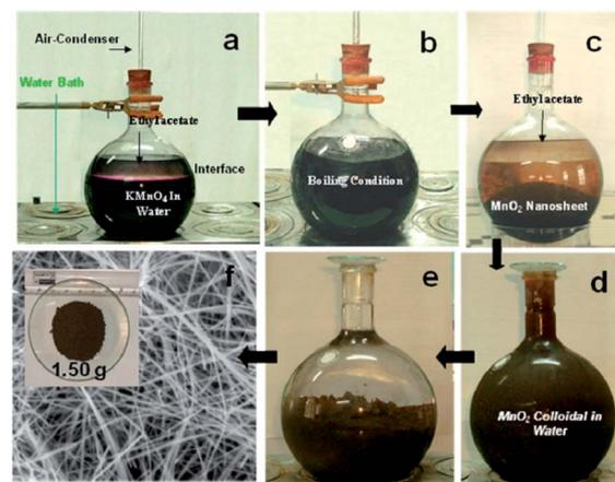
Fig. 2 Preparation of gram level  $\alpha$ - $\text{MnO}_2$  nanowires from aqueous  $\text{KMnO}_4$ /ethyl acetate biphasic system and their different stages (a–f) in digital/FESEM images. Reproduced by Sinha *et al.*<sup>65</sup> with permission from ACS.
