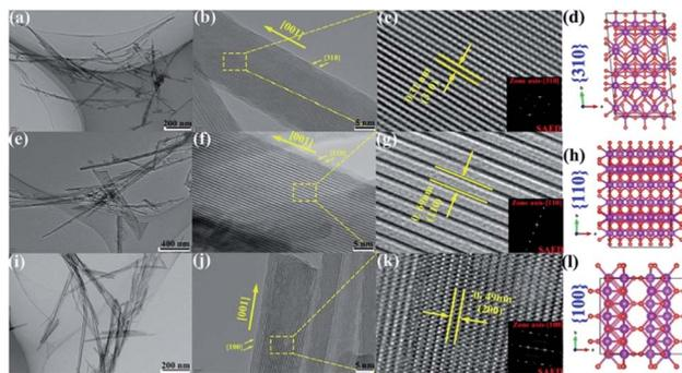
Fig. 6 TEM and HRTEM images of (a–c)  $\alpha$ -MnO<sub>2</sub>-310, (e–g)  $\alpha$ -MnO<sub>2</sub>-110, and (i–k)  $\alpha$ -MnO<sub>2</sub>-100. Atomic structure of the (d) {310}, (h) {110}, and (l) {100} surface of  $\alpha$ -MnO<sub>2</sub>. Small (red) spheres are oxygen and large (purple) are manganese. Reproduced by Rong *et al.*<sup>86</sup> with permission from ACS.
