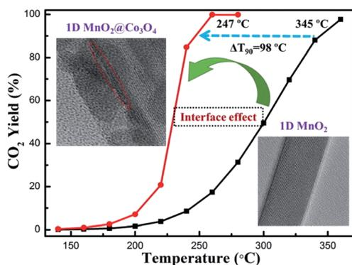
Fig. 11 Benzene oxidation activity tests of the 1D MnO<sub>2</sub>@Co<sub>3</sub>O<sub>4</sub> and 1D MnO<sub>2</sub> catalysts. Reproduced by Tang *et al.*<sup>31</sup> with permission from Elsevier.
