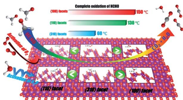
Fig. 7  $\alpha$ -MnO<sub>2</sub> nanowires with (100), (110) and (310) facets for HCHO oxidation. Reproduced by Rong *et al.*<sup>86</sup> with permission from ACS.
