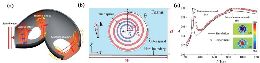
Fig. 3 Schematic of the structure of acoustic metamaterials based on porous media. (a) Schematic of common sound energy dissipation mechanisms in a porous sound-absorbing material.<sup>58</sup> (b) The 2D cross section of the dual-spiral structure.<sup>68</sup> (c) The sound absorption coefficient from the simulation and the experiment of the dual-spiral structure; the insets are the simulated acoustic field distributions.<sup>68</sup>
