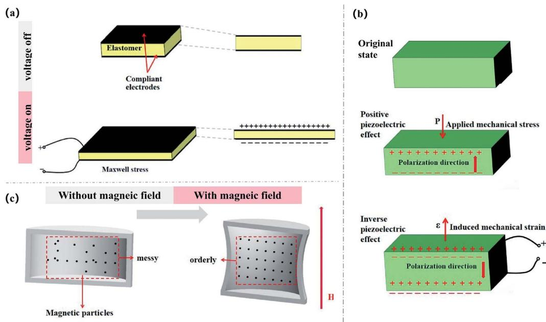
Fig. 6 Schematic for the working principle of some intelligent materials utilized in acoustic structures. (a) Dielectric elastomer, (b) polyvinylidene fluoride actuator, (c) magnetorheological elastomer.
