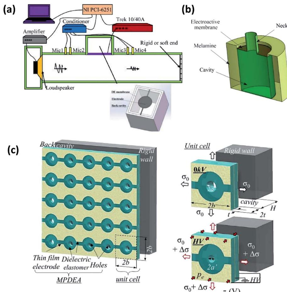
Fig. 7 (a) Experimental setup for the tunable silencer based on DE actuator.<sup>96</sup> (b) 3D schematic of the Helmholtz resonator components with DE membrane.<sup>41</sup> (c) A broader band acoustic absorber using DE actuators with MPP structure: an array of electrically tunable holes in DE actuators (left); its unit cell with a hole at either passive or active states (right).<sup>97</sup>
