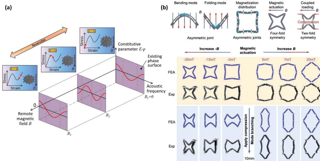
Fig. 9 (a) Conceptual schematics of study:<sup>117</sup> the magnetically induced lattice buckling was harnessed to enable tunable sign of effective modulus  $E$  between positive and negative. (b) The metamaterial unit cell design and the concept of deformation mode branching.<sup>118</sup>
