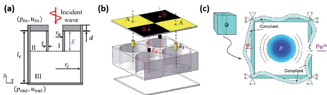
Fig. 1 Helmholtz resonance structures. (a) The cross-sectional view of a Helmholtz resonator unit with an extended neck.<sup>44</sup> (b) Schematic of a checkerboard absorber composed of alternating resonators A and B with varying-length extended necks.<sup>44</sup> (c) Schematic of the complete compliant-material resonator and a cross-section.<sup>46</sup>
