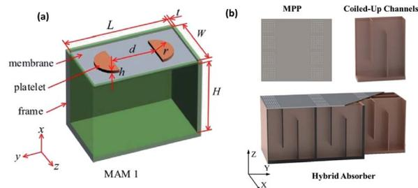
Fig. 4 (a) Schematic of a membrane-type metamaterial.<sup>72</sup> (b) Schematic of the hybrid metamaterial absorber composed of a micro-perforated panel (MPP) as a top face sheet and coiled-up Fabry–Pérot channels with folding number  $n$ . The front wall is cut off to see the details inside.<sup>75</sup>
