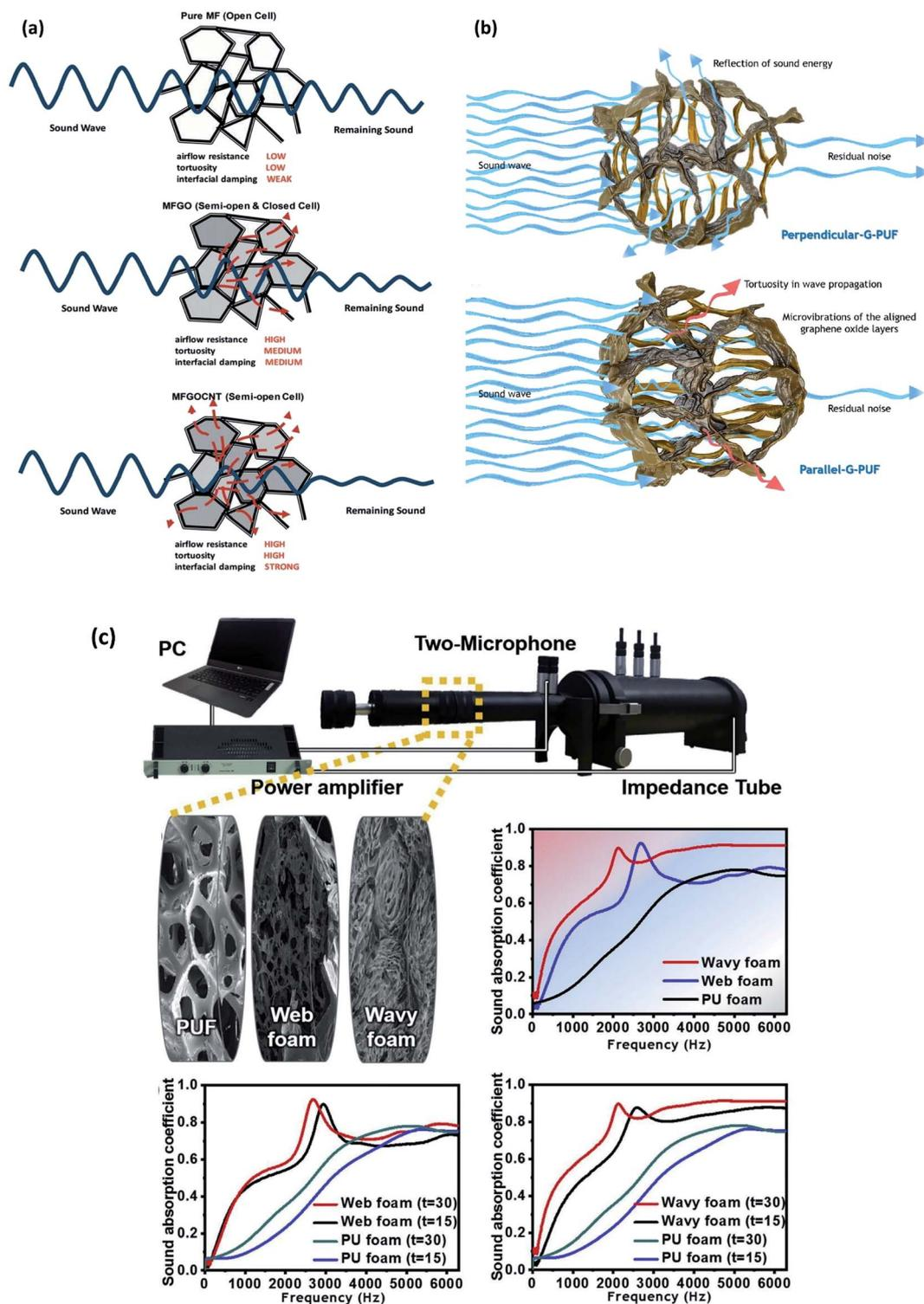
Fig. 10 (a) Schematic of acoustic propagation through pure melamine foams, melamine foam with GO, melamine foam with GO and CNT.<sup>129</sup> (b) Schematic of the mechanism of sound absorption in a directionally antagonistic graphene sound absorber.<sup>130</sup> (c) Schematic of a 29 mm diameter of the polyurethane foam, the web foam, and the wavy foam. And Comparison of sound absorption performance for the three samples.<sup>131</sup>
