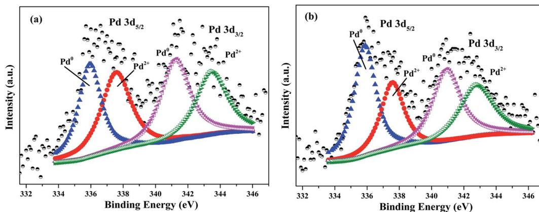
Fig. 3 Pd 3d XPS spectra of (a) Pd/AC and (b) Pd/N<sub>AC</sub>.
