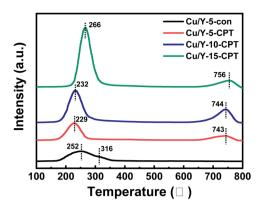
Fig. 6 H<sub>2</sub>-TPR profile of Cu/Y-5-con and Cu/Y-x-CPT (x = 5-15 wt%).
