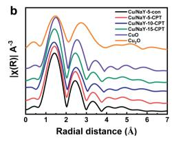
Fig. 7 Normalized Cu K-edge XANES spectra (a) and magnitude of FourierFourier transformed EXAFS spectra (b) of Cu/Y catalysts along with the  $Cu^{2+}$  and  $Cu^{+}$  reference compounds (CuO and  $Cu_{2}O$ ). The spectra are displaced vertically for clarity.
