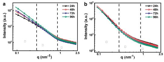
Fig. 3 Scattering curves of sol-con (a) and sol-CPT-1.0 (b) samples under different aging times
