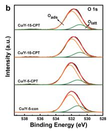
Fig. 8 X-ray photoelectron spectra for Cu 2p (a) and O 1s (b) of Cu/Y catalysts.
