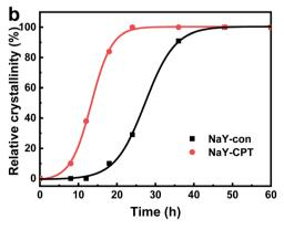
Fig. 1 XRD patterns (a) and crystallization curves (b) of NaY-con and NaY-CPT under different crystallization times.
