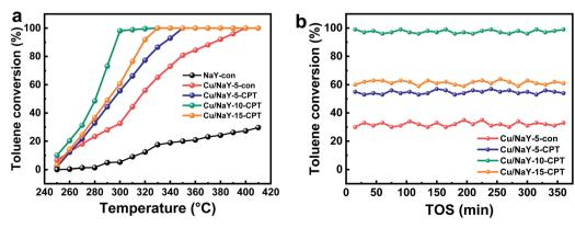
Fig. 9 Catalytic activity as a function of temperature (a) and time on stream at 300 °C (b) for Cu/Y catalysts.
