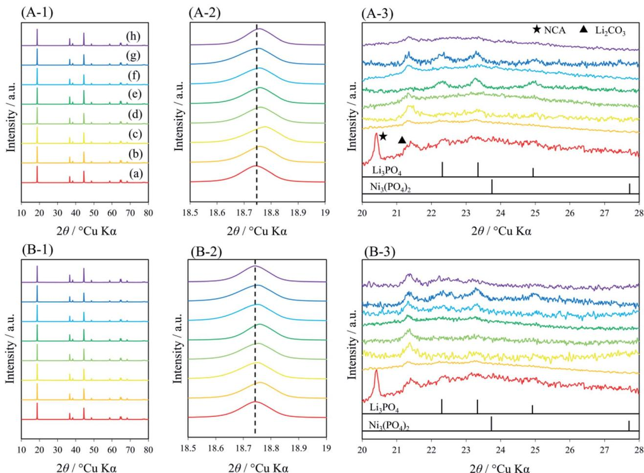
Fig. 6 pXRD patterns of (a) pristine NCA and (b–h) coated NCA with standard peak patterns of  $\text{Li}_3\text{PO}_4$  (JCPDS 83-0339) and  $\text{Ni}_3(\text{PO}_4)_2$  (JCPDS 46-1388). Sample (b) was not heat-treated, and samples (c–h) were heat-treated at (c) 200, (d) 250, (e) 300, (f) 350, (g) 400 and (h) 450 °C in (A) Ar and (B) air atmospheres.
