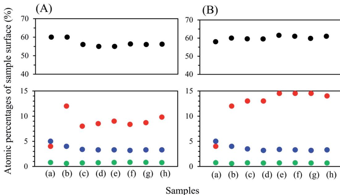
Fig. 4 Atomic percentage on the surface of samples evaluated with XPS. (a) Pristine NCA and (b–h) coated NCA samples. (b)  $\text{Li}_3\text{PO}_4$ -coated NCA samples without heat treatment, (c–h) coated NCA with heat treatment. Temperature of heat treatment: (c) 200, (d) 250, (e) 300, (f) 350, (g) 400 and (h) 450 °C. Atmosphere for heat-treatment: (A) Ar and (B) air. ●: oxygen, ●: nickel, ●: lithium, ●: phosphorus.
