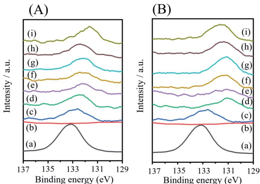
Fig. 5 XPS spectral profiles in the P 2p region of (a)  $\text{Li}_3\text{PO}_4$  powder, (b) pristine NCA and (c–i) coated NCA. Sample (c) was not heat-treated, and samples (d–i) were heat-treated at (d) 200, (e) 250, (f) 300, (g) 350, (h) 400 and (i) 450 °C in (A) Ar and (B) air atmospheres.
