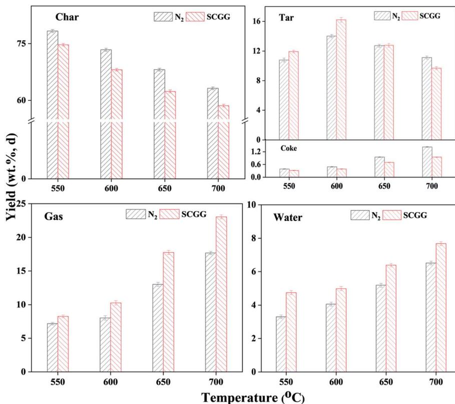
Fig. 3 Yields of pyrolysis products under N<sub>2</sub> and SCGG at different temperatures.
