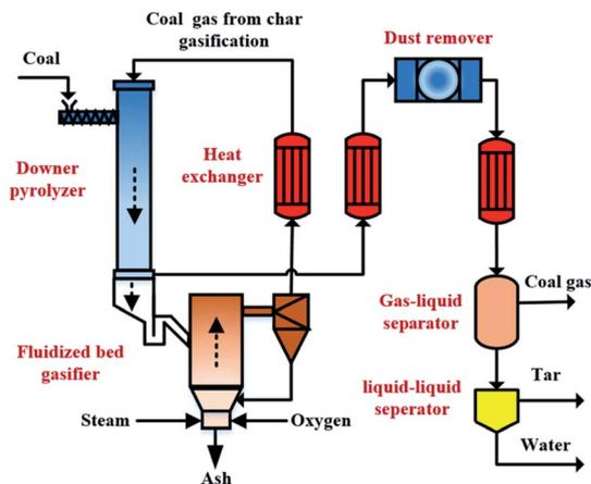
Fig. 1 Principle of the novel poly-generation process.
