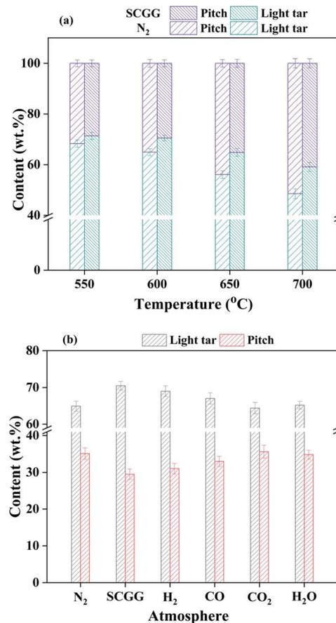
Fig. 6 Fraction distribution of tar under N<sub>2</sub> and SCGG at different temperatures (a) and under individual gas at 600 °C (b).
