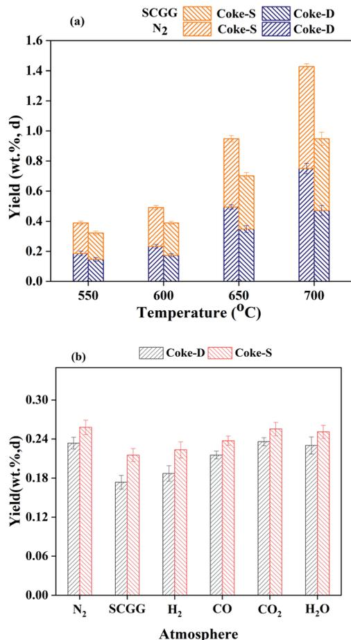
Fig. 5 Yields of coke-S and coke-D under N<sub>2</sub> and SCGG at different temperatures (a) and under individual gas at 600 °C (b).
