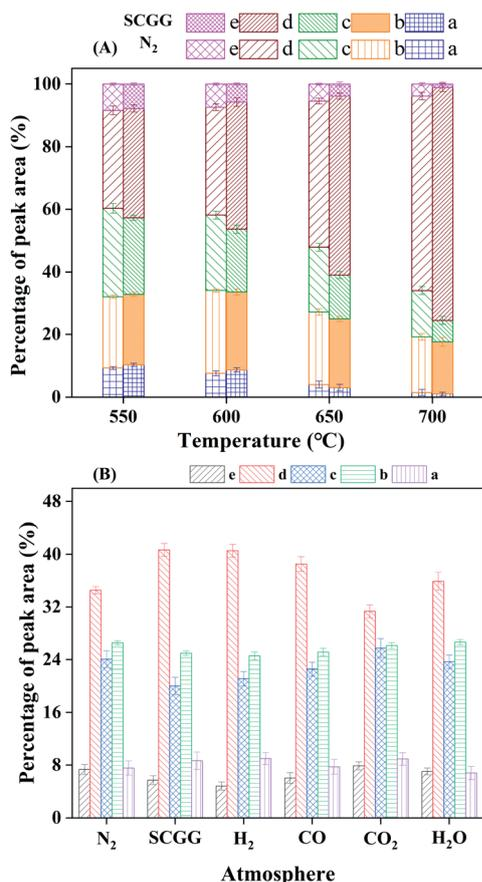
Fig. 7 Chemical composition of tar under N<sub>2</sub> and SCGG at different temperatures (A) and under individual gas at 600 °C (B) ((a) aliphatics, (b) phenols, (c) oxygenated compounds, (d) aromatics, (e) heterocyclic compounds).
