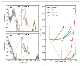
Fig. 3 Transmission spectra for T–H heterophase junction of MoS $_2$  monolayer containing various sulfur vacancies at both interfaces at (a) bias  $=0.00\,\text{V}$  and (b) bias  $=1.40\,\text{V}$ . Energies are shifted with respect to their corresponding Fermi energy. The insets show the change in the electronic transmission channels at the top of the valence band. (c) I-V characteristics for the same devices. The inset shows the current around the threshold voltage.
