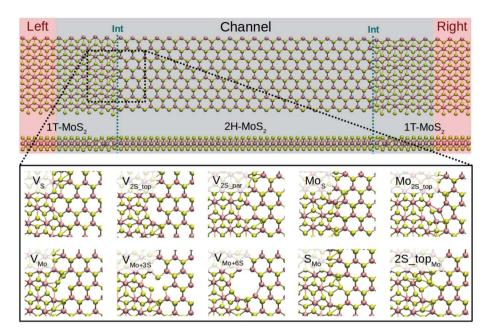
Fig. 1 (Upper) Schematic of the T-H heterophase junction of  $MoS_2$  monolayer. Electrodes (only  $1T-MoS_2$ ) and channel region (a combination of  $1T-MoS_2$ ) are highlighted with shaded red and black, respectively. The interfaces are indicated with green dashed-lines. (Lower) Optimized structures of the point defects at the left interface of the devices are shown. Only defects at the left electrode are shown here. The complete devices are shown in Fig. S1 in the ESI.†
