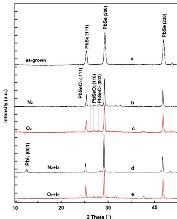
Fig. 2 XRD patterns of PbSe films. (a) As-grown, and sensitized at (b) pure N<sub>2</sub>, (c) pure O<sub>2</sub>, (d) N<sub>2</sub>/I<sub>2</sub>, and (e) O<sub>2</sub>/I<sub>2</sub>.
