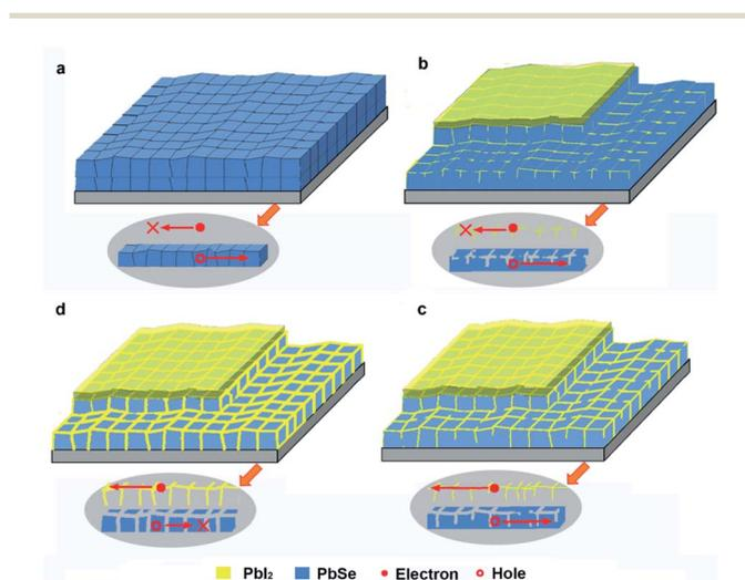
Fig. 6 The schematic of the N<sub>2</sub>/I<sub>2</sub> sensitization process and the photo-generated electrons and holes transporting channels at various sensitization time. (a) As-grown, (b) initial, (c) optimized and (d) over sensitization stages.
