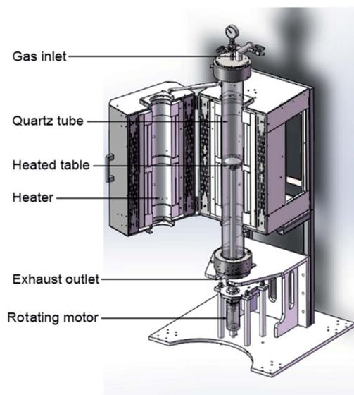
Fig. 1 Schematic diagram of a homemade sensitization setup.
