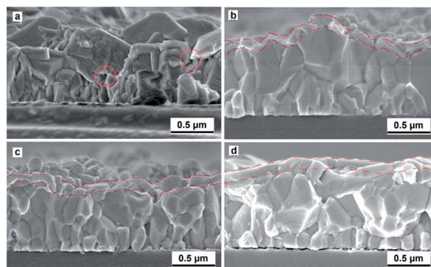
Fig. 3 FESEM images of PbSe films. (a) The as-grown film and the film sensitized in (b) N<sub>2</sub>, (c) N<sub>2</sub>/I<sub>2</sub> and (d) O<sub>2</sub>/I<sub>2</sub>.
