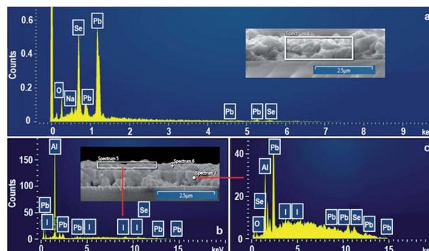
Fig. 4 EDS spectra of the PbSe films. (a) As-grown and (b) top-layer and (c) bottom layer of sensitized PbSe film under N<sub>2</sub>/I<sub>2</sub> atmosphere.
