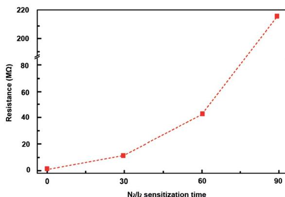
Fig. 5 The dependence of N<sub>2</sub>/I<sub>2</sub> sensitization on the resistance of PbSe detectors.
