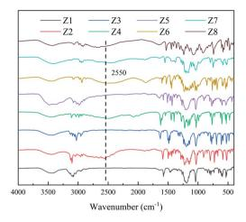
Fig. 2 IR spectra of Zwitterions.
