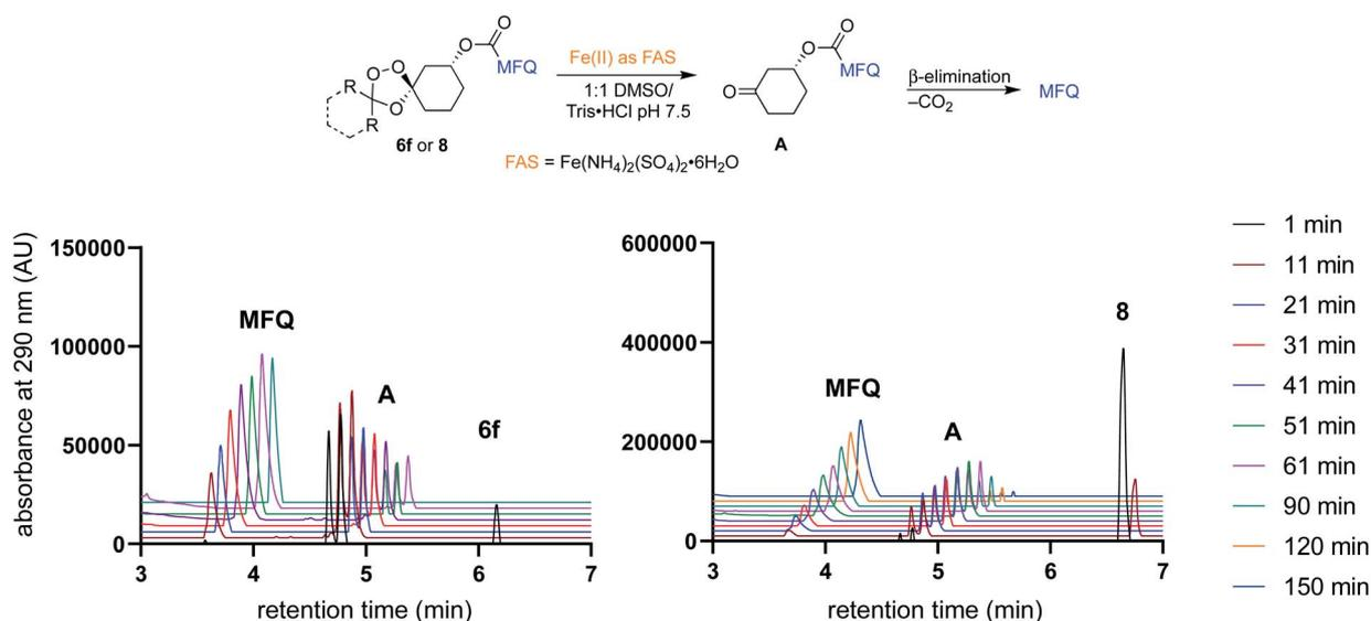
**Fig. 2** *In vitro* iron fragmentation studies of the previously described, *in vivo* efficacious mefloquine conjugate **8** and the new congener **6f** bearing a bicyclo[2.1.1]heptane ring in place of the adamantane. Fragmentation of the trioxolane with FAS is rapid for both conjugates, with  $\beta$ -elimination from common intermediate **A** being the rate limiting step in mefloquine (MFQ) release.
