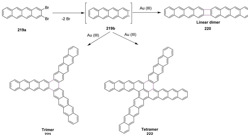
Scheme 94 On-surface cyclization of *o*-dihalotetracenes to four and six-membered rings.
