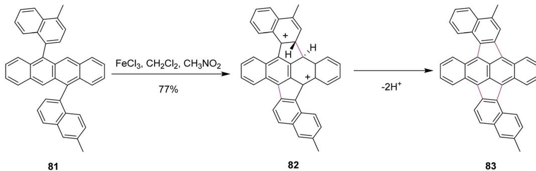
Scheme 34 Twofold Scholl cyclization by  $\text{FeCl}_3$ .
