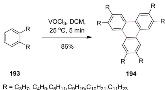
Scheme 83 Synthesis of triphenylenes with vanadium oxytrichloride.
