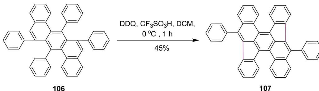
Scheme 44 Synthesis of fullerene pentagons with DDQ.
