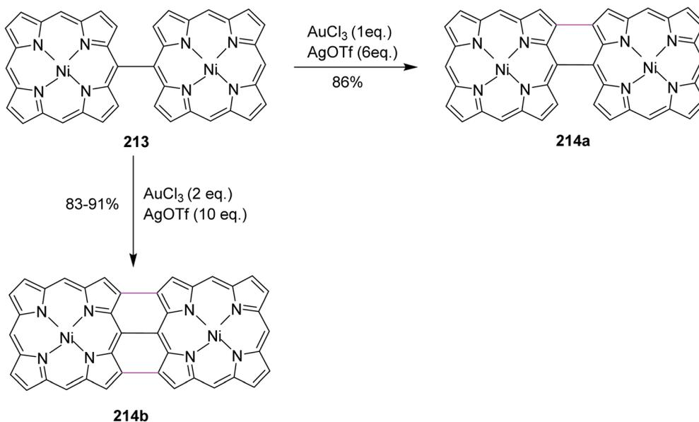
Scheme 91 C–C coupling of porphyrin units using Au(III).
