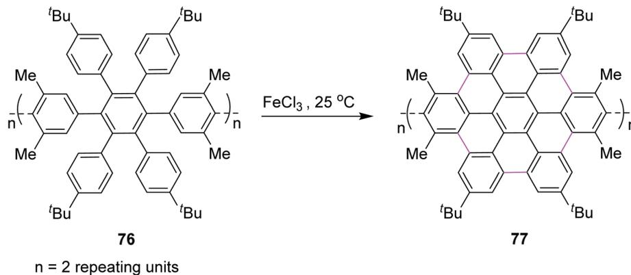
Scheme 32 Cyclodehydrogenation of polyphenylenes by  $\text{FeCl}_3$ .
