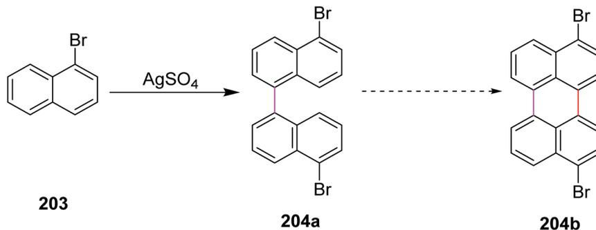
Scheme 88 C–C coupling of naphthalene units with  $\text{AgSO}_4$ .
