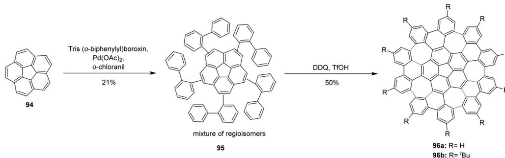
Scheme 40 DDQ-induced synthesis of grossly-warped graphene molecules.
