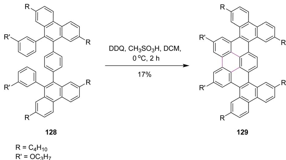
Scheme 51 Synthesis of nanographene unit *via* the Scholl reaction.
