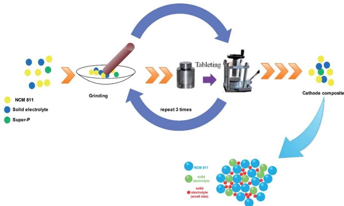
Fig. 1 The schematic diagram for the cathode composite preparation process.
