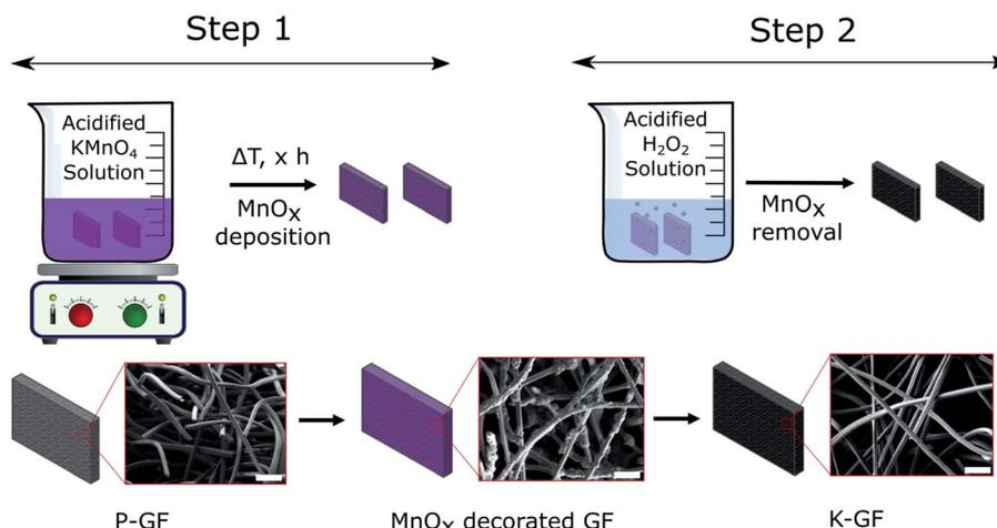
**Fig. 1** Schematic diagram of the K-GF fabrication process. Step 1 involves the deposition of MnO<sub>x</sub> layers onto the P-GF electrode surface using acidified KMnO<sub>4</sub> solutions. Step 2 involves the removal of MnO<sub>x</sub> layers using an acidified H<sub>2</sub>O<sub>2</sub> solution to produce the K-GF electrode. SEM images depict the fibre morphology during each stage of the fabrication process. The scale bars in each SEM image represent 50 μm.
