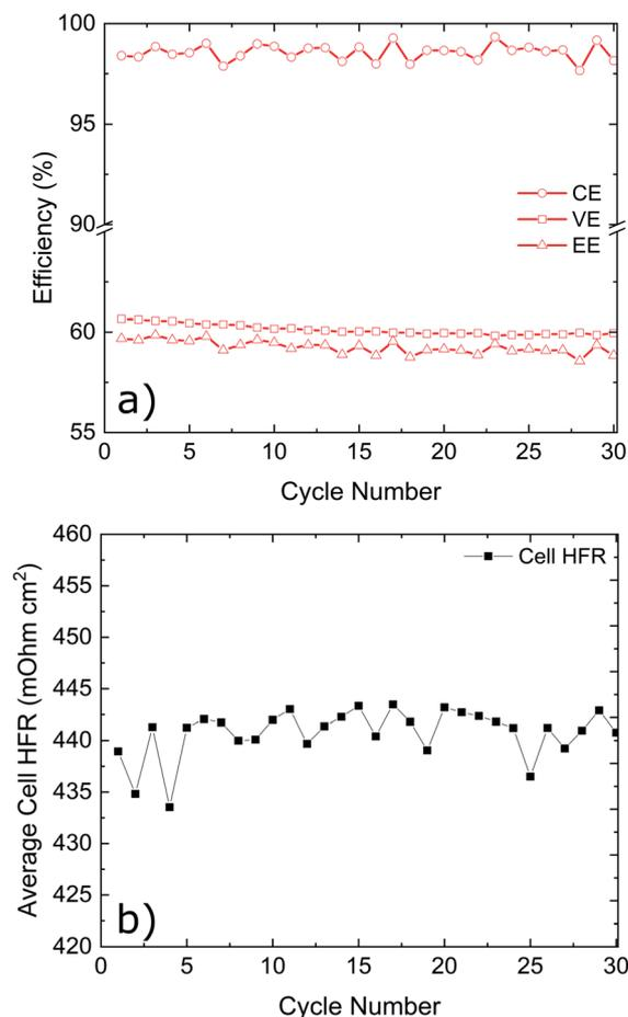
Fig. 7 K-GF electrode cycling at  $400 \text{ mA cm}^{-2}$  for 30 cycles. (a) CE, EE and VE values for the K-GF electrode cycled at  $400 \text{ mA cm}^{-2}$  for 30 cycles. (b) Average cell HFR values of the system during cycling.
