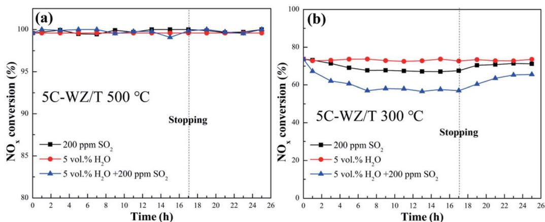
Fig. 2 NO conversion of 5C-WZ/T in the presence of 5 vol% H<sub>2</sub>O, 200 ppm SO<sub>2</sub> and 200 ppm SO<sub>2</sub> + 5 vol% H<sub>2</sub>O at 15 000 h<sup>-1</sup>. (a) 5C-WZ/T at 500 °C, (b) 5C-WZ/T at 300 °C.
