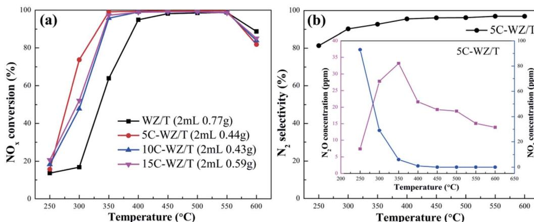
Fig. 1 (a)  $\text{NO}$  conversion of different catalysts; (b)  $\text{N}_2$  selectivity of 5C-WZ/T catalyst. Reaction condition: 500 ppm NO, 500 ppm  $\text{NH}_3$ , 10%  $\text{O}_2$ , GHSV of 15 000  $\text{h}^{-1}$  and  $\text{N}_2$  balance gas.
