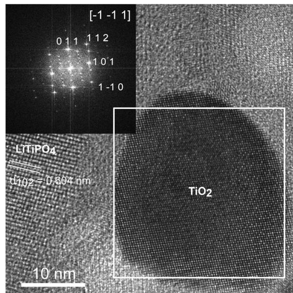
**Fig. 4** HRTEM image of a nanoparticle in zone axis orientation. The FFT generated from the white box is shown at the inset and can be indexed as  $[-1 -1 1]$  zone axis of anatase phase of  $\text{TiO}_2$  (ICSD #9852). In the neighbouring grain lattice plane fringes with a distance of 6.04 Å are observed, which match well with  $\{1 0 2\}$ -planes of the  $R3c$  structure of LTP (ICSD #95979).
