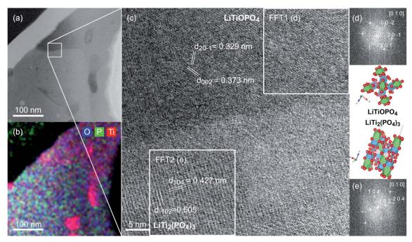
Fig. 5 (a) STEM-HAADF image and (b) STEM-EDS map of a boundary between LiTiOPO<sub>4</sub> and LiTi<sub>2</sub>(PO<sub>4</sub>)<sub>3</sub>. The box in (a) marks the area from which the HRSTEM image in (c) was recorded with both phases being in zone axis orientation as indexed in the FFTs shown in (d) (LiTiOPO<sub>4</sub>) and (e) (LiTl<sub>2</sub>(PO4)<sub>3</sub>) generated from the areas marked by the white squares.
