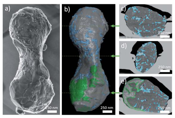
Fig. 6 (a) Top view SE image of the particle selected for FIB tomography. (b) Surface rendering of the segmented FIB tomography data. Grey, green and blue colours represent LTP, LiTiOPO<sub>4</sub> and  $TiO_2$  respectively. The red arrows indicate the positions of the slices shown in (c)–(e) visualizing the segmentation inside the volume.
