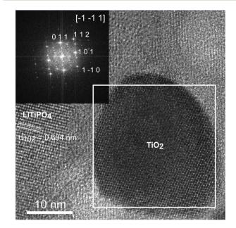
Fig. 4 HRTEM image of a nanoparticle in zone axis orientation. The FFT generated from the white box is shown at the inset and can be indexed as  $[-1 - 1 \ 1]$  zone axis of anatase phase of TiO<sub>2</sub> (ICSD #9852). In the neighbouring grain lattice plane fringes with a distance of 6.04 Å are observed, which match well with  $\{1 \ 0 \ 2\}$ -planes of the R3c structure of LTP (ICSD #95979).
