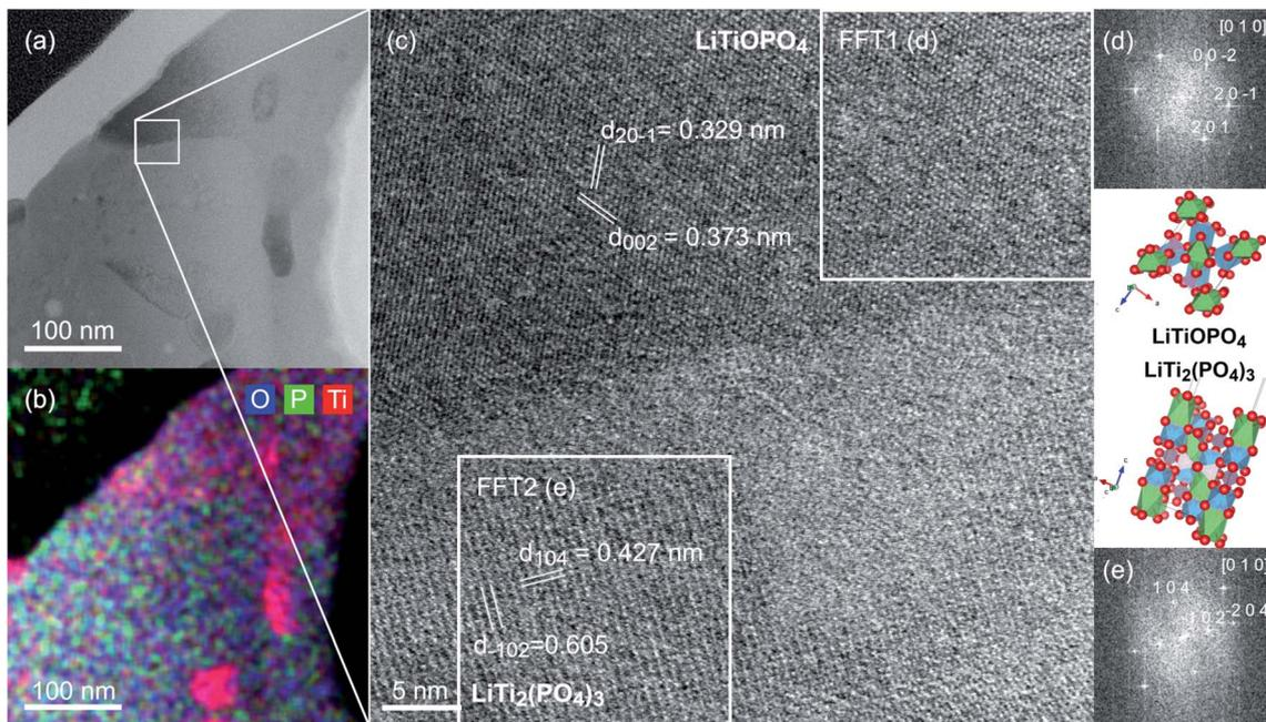
Fig. 5 (a) STEM-HAADF image and (b) STEM-EDS map of a boundary between  $\text{LiTiOPO}_4$  and  $\text{LiTi}_2(\text{PO}_4)_3$ . The box in (a) marks the area from which the HRSTEM image in (c) was recorded with both phases being in zone axis orientation as indexed in the FFTs shown in (d) ( $\text{LiTiOPO}_4$ ) and (e) ( $\text{LiTi}_2(\text{PO}_4)_3$ ) generated from the areas marked by the white squares.
