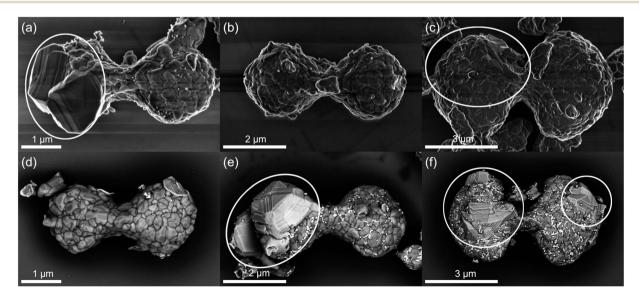
Fig. 1 SEM micrographs of spindle like particles of different sizes: small ((a) and (e)), medium ((b) and (d)) and large ((c) and (f)). Regions with different morphology indicating the presence of a secondary phase are marked in (a), (c), (e) and (f).
