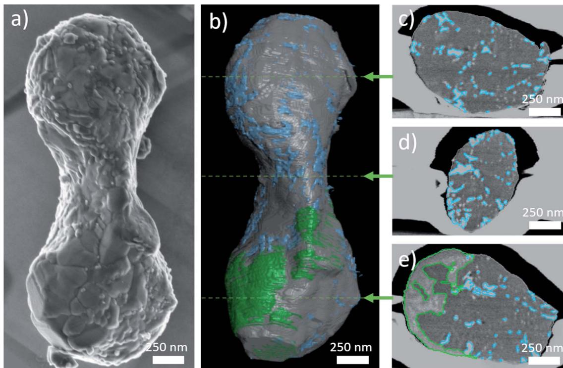
Fig. 6 (a) Top view SE image of the particle selected for FIB tomography. (b) Surface rendering of the segmented FIB tomography data. Grey, green and blue colours represent LTP,  $\text{LiTiOPO}_4$  and  $\text{TiO}_2$  respectively. The red arrows indicate the positions of the slices shown in (c)–(e) visualizing the segmentation inside the volume.
