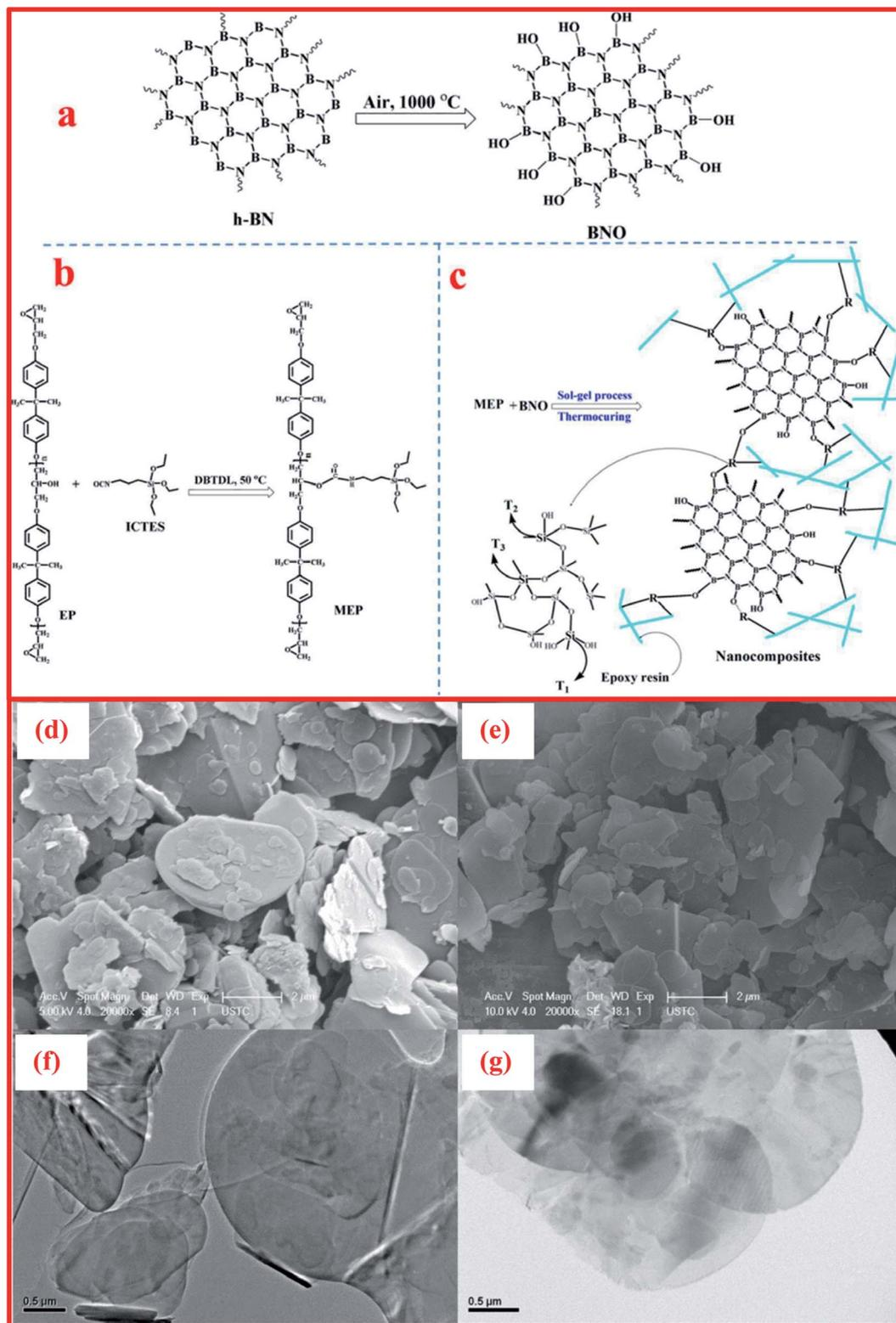
Fig. 10 Illustrations of the synthesis processes of (a) BNO, (b) MEP, and (c) BNO/MEP nanocomposites, SEM images of (d) h-BN and (e) BNO, and TEM micrographs of (f) h-BN and (g) BNO.<sup>126</sup>
