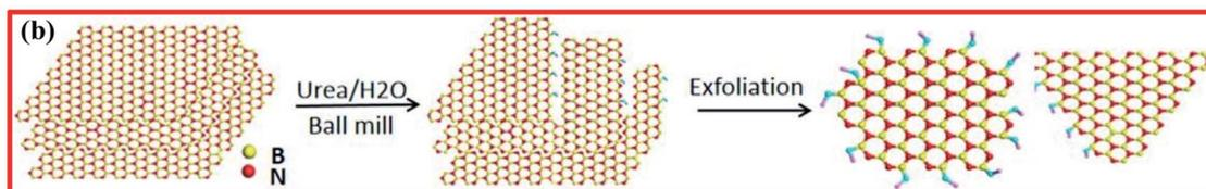
Fig. 7 (a) A flow chart showing the synthesis of small-layer BN and large-layer BN and (b) a schematic illustration of the exfoliation process using a ball-milling technique.<sup>121</sup>
