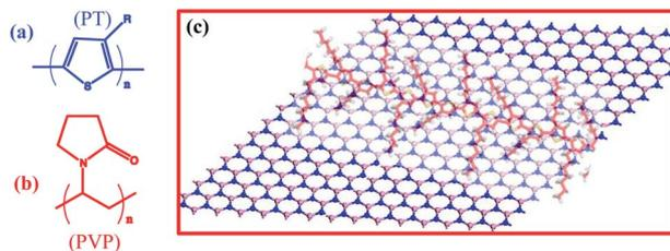
Fig. 21 (a) The structure of polythiophene (PT), (b) the structure of polyvinylpyrrolidone (PVP), and (c) a schematic model of the  $\pi$ - $\pi$  stacking between BNNSs and polythiophene (PT).<sup>215</sup>
