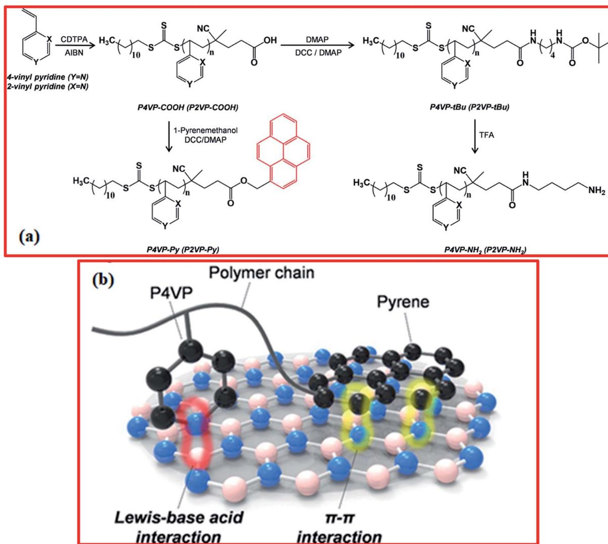
Fig. 27 (a) The reaction scheme for P<sub>n</sub>VP (n = 2 and 4) with different functional groups: carboxylic acid (P<sub>n</sub>VP-COOH), pyrene (P<sub>n</sub>VP-Py), tert-butyl (P<sub>n</sub>VP-tBu), and amine (P<sub>n</sub>VP-NH<sub>2</sub>). (b) An illustration of the suggested mechanism for dual Lewis acid–base and  $\pi - \pi$  interactions using P4VP-Py molecules on BN.<sup>237</sup>
