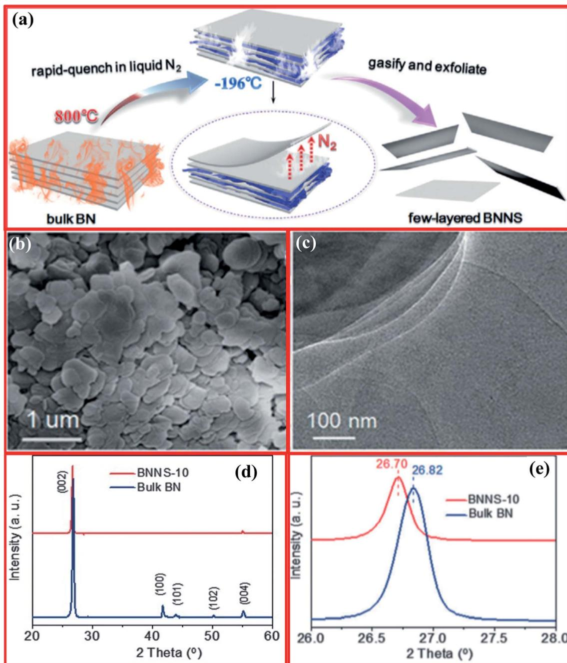
Fig. 12 (a) The gas exfoliation of h-BN triggered via thermal expansion, (b) an SEM image of BNNS-10, (c) a TEM image of BNNS-10, and (d and e) structural characterization of bulk h-BN and BNNS-10.<sup>128</sup>
