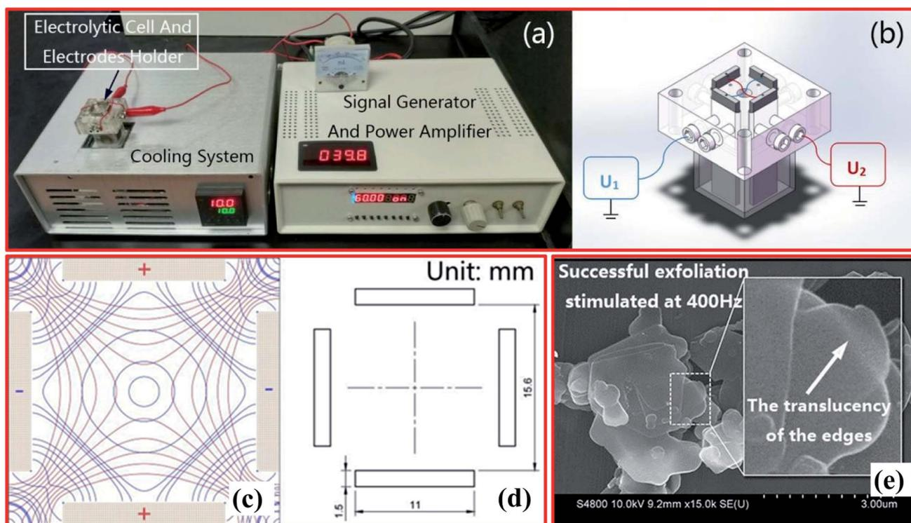
Fig. 13 (a) The assembly of the electrical stimulation system. (b) The quadrupole electrolytic cell ( $U_1$  and  $U_2$  are differential amplification voltages). (c) The rectangular quadrupole electric field (the red lines represent potential lines, and the blue lines represent field intensity lines). (d) The sizes and positions of the orthogonal titanium electrodes. (e) An SEM image of h-BN exfoliated at the optimal frequency of 400 Hz.<sup>132</sup>
