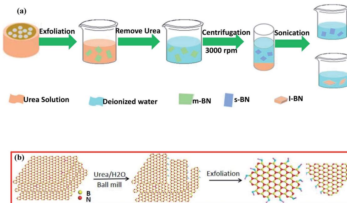
Fig. 7 (a) A flow chart showing the synthesis of small-layer BN and large-layer BN and (b) a schematic illustration of the exfoliation process using a ball-milling technique.<sup>121</sup>
