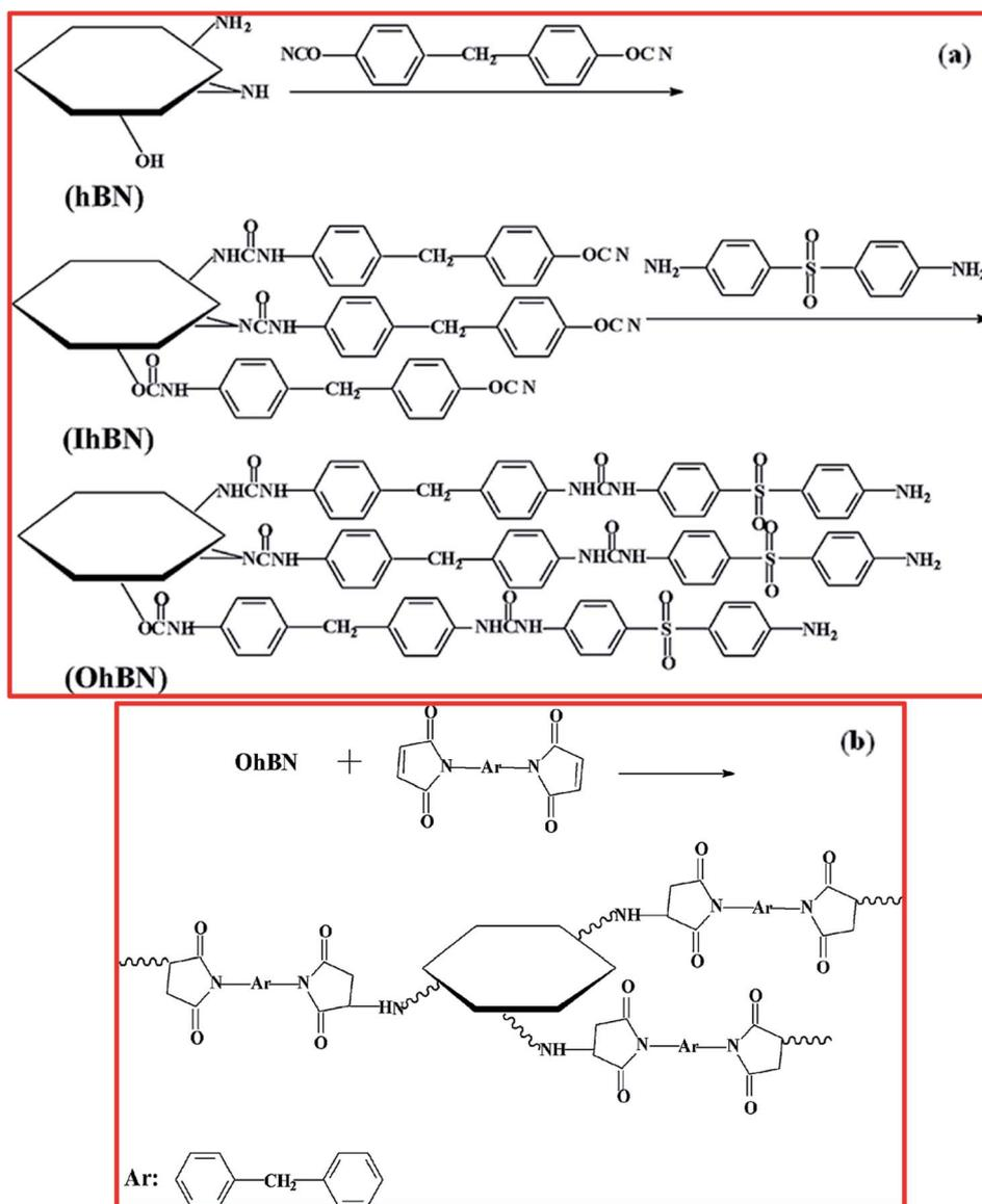
Fig. 19 (a) The surface treatment of h-BN and (b) the reactions between h-BN and BDM.<sup>183</sup>
