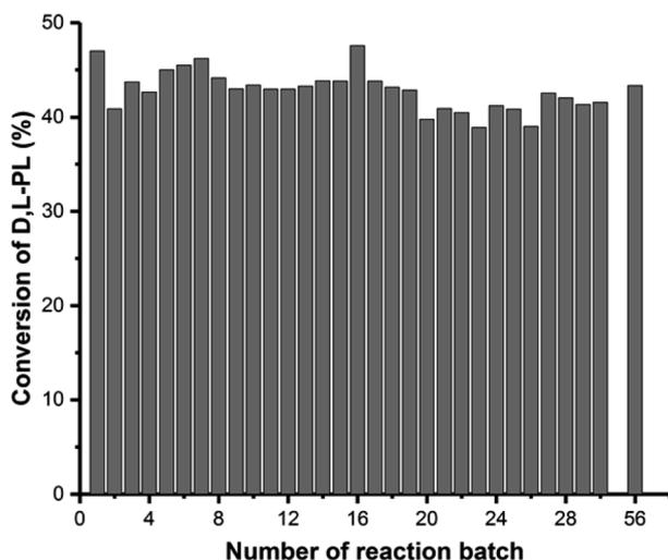
Fig. 4 Repeated batch reactions for industrial kinetic resolution of  $D,L$ -PL with immobilized cell.
