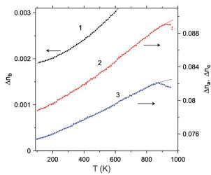
Fig. 8 Temperature dependences of the birefringence of LiGaS $_2$  at a wavelength of about 400 nm: (1)  $\Delta n_{\rm b}$ , (2)  $\Delta n_{\rm c}$ , (3)  $\Delta n_{\rm a}$ .
