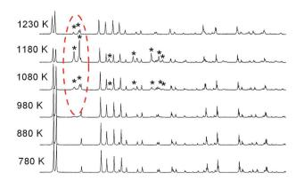
Fig. 6 A series of X-ray diffractograms of the LiGaS $_2$  sample obtained in a high vacuum ( $\sim$ 5 × 10 $^{-4}$  mBar) at temperatures in the range of 780–1230 K. The dotted line shows the most intense reflexes related to the oxygen-containing phase. On the diffractogram obtained at T=1080 K, all reflexes related to this phase, supposedly LiGaO $_{2-x}S_x$ , are marked with asterisks.
