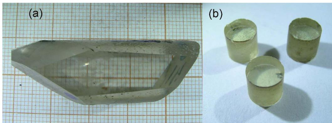
Fig. 1 The image of the LiGaS<sub>2</sub> boule (a) and the LiGaS<sub>2</sub> cylinders (b) with axes along different crystallographic directions for measuring the thermal conductivity and the isotropic point.
