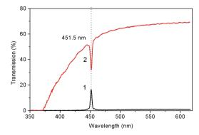
Fig. 10 Transmission spectra for (100) LiGaS $_2$  plate with a thickness of 5 mm placed between crossed (1) and parallel (2) film polarizers.
