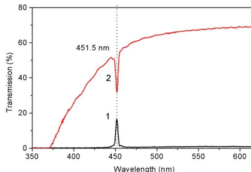
Fig. 10 Transmission spectra for (100) LiGaS<sub>2</sub> plate with a thickness of 5 mm placed between crossed (1) and parallel (2) film polarizers.
