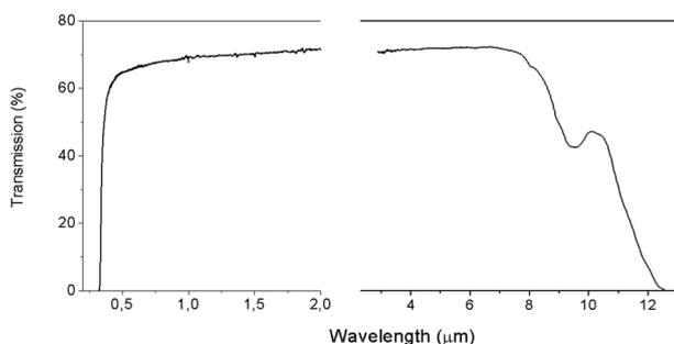
Fig. 2 Room-temperature transmission spectrum for a 2 mm thick plate cut from as grown LiGaS<sub>2</sub>.
