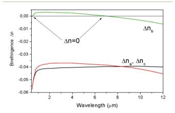
Fig. 9 Dependence of the birefringence  $\Delta n$  on the wavelength for LiGaS<sub>2</sub>. The arrows show two isotropic points, where  $\Delta n=0$ .
