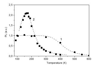
Fig. 15 The temperature dependence of the integral PL in the bands of about 600 nm (1) and 425 nm (2) in LiGaS<sub>2</sub> at excitation of 300 and 375 nm, respectively. The dots represent the experimental data, while the dotted curves show the results of calculations according to eqn (3) with the parameters  $\Delta E = 0.14$  eV,  $\tau_R \nu_0 = 4 \times 10^3$  (1) and  $\Delta E = 0.35$  eV,  $\tau_R \nu_0 = 1.7 \times 10^4$  (2).
