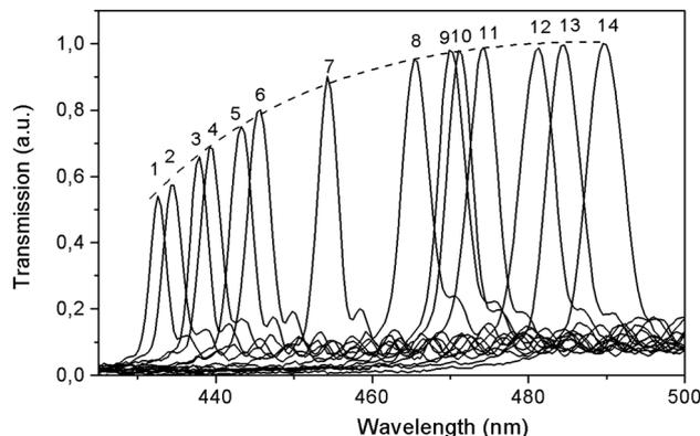
Fig. 11 Transmission spectra for a (100) LiGaS<sub>2</sub> plate 5 mm thick placed between the crossed polarizers. Spectra were measured at fourteen different temperatures in the temperature range of 77 K (curve (1)) to 550 K (14).
