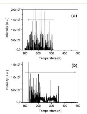
Fig. 17 Temperature dependence of spontaneous luminescence in  $LiGaS_2$  in the cooling (a) and heating (b) modes.
