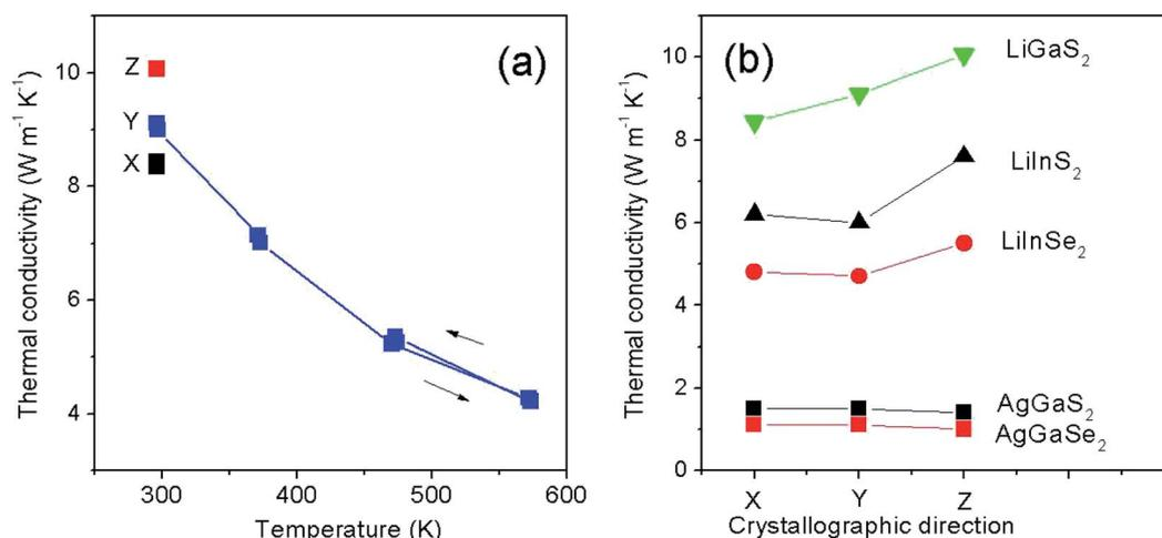
Fig. 7 Thermal conductivity for chalcogenides: (a) LiGaS<sub>2</sub> along *X*, *Y* and *Z* directions at room temperature and temperature dependence for  $\chi_Z$  in the 300 to 557 K range. Arrows indicate heating or cooling regime. (b) Comparison of values for commercial AgGaS<sub>2</sub>, AgGaSe<sub>2</sub> and for crystals of the LiBC<sub>2</sub> family with B = In, Ga and C = S, Se.
