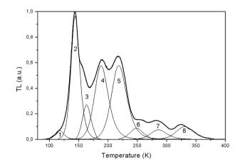
Fig. 16 TL curve for LiGaS $_2$  after 365 nm excitation at 80 K and the results of deconvolution into 8 components (shown in thin lines). The resulting parameters for the corresponding capture centers are shown in the Table 3 below.
