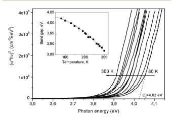
Fig. 13 Absorption spectra for LiGaS<sub>2</sub> in the region of the fundamental absorption edge, measured at 12 different temperatures in the range from 77 to 300 K and presented in coordinates  $(\alpha h \nu)^2 = f(h \nu)$  (Tauc plot). The insert shows the temperature dependence for the band gap in LiGaS<sub>2</sub>. The points are obtained experimentally, while the line shows the result of the approximation in accordance with the Varshni equation.<sup>21</sup>
