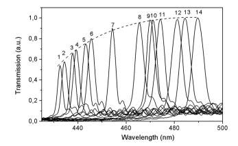
Fig. 11 Transmission spectra for a (100) LiGaS $_2$  plate 5 mm thick placed between the crossed polarizers. Spectra were measured at fourteen different temperatures in the temperature range of 77 K (curve (1)) to 550 K (14).
