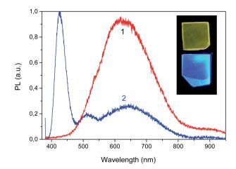
Fig. 14 PL spectra recorded at T=80 K, at 300 nm (1) and 375 nm (2) excitation for LiGaS<sub>2</sub> annealed in vacuum. The insert shows the room temperature PL patterns obtained at UV excitation with 300 nm light (upper image with orange emission) and 375 nm (lower image with blue PL).
