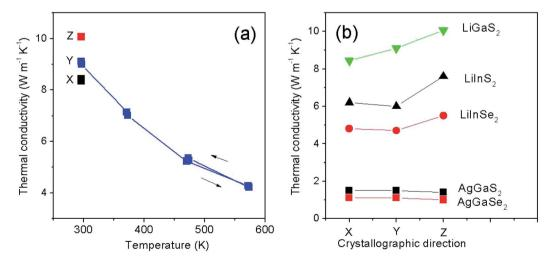
Fig. 7 Thermal conductivity for chalcogenides: (a) LiGaS<sub>2</sub> along X, Y and Z directions at room temperature and temperature deendence for  $\chi_Z$  in the 300 to 557 K range. Arrows indicate heating or cooling regime. (b) Comparison of values for commercial AgGaS<sub>2</sub>, AgGaSe<sub>2</sub> and for crystals of the LiBC<sub>2</sub> family with B = In, Ga and C=S, Se.
