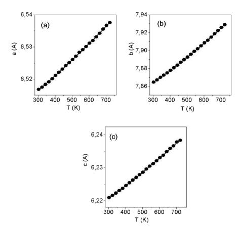
Fig. 5 Thermal dependences of cell parameters a (a), b (b) and c (c) of LiGaS<sub>2</sub>.
