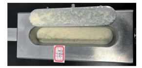
Fig. 5 Proppant cell in the conductivity test device
