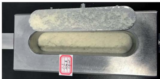
Fig. 5 Proppant cell in the conductivity test device.
