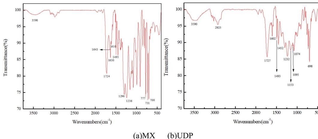
Fig. 7 FT-IR spectra of UDP.
