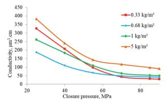
Fig. 19 Conductivity test results under different concentrations.
