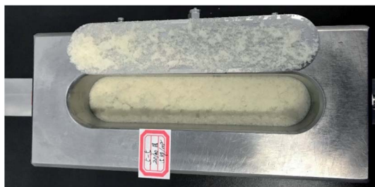
Fig. 5 Proppant cell in the conductivity test device.
