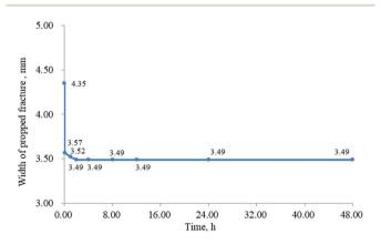
Fig. 18 Width of propped fracture at different time.
