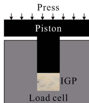
Fig. 4 Experimental device to test the compressive strength.
