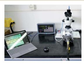
Fig. 2 Image collecting microscope.
