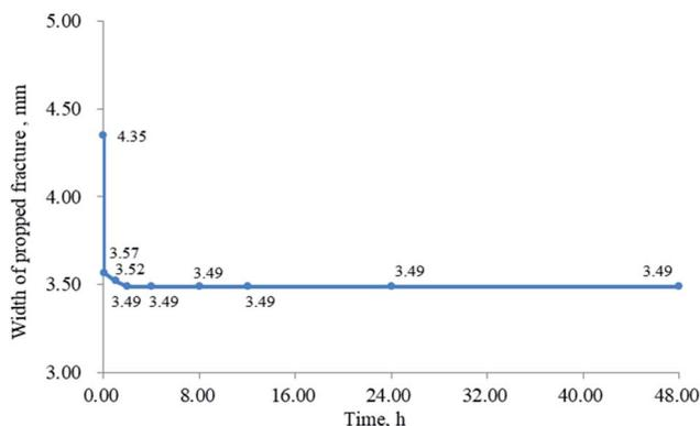
Fig. 18 Width of propped fracture at different time.
