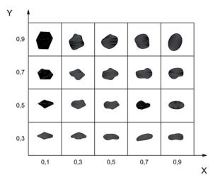
Fig. 3 Chart for visual estimation of sphericity and roundness in ISO 13503-2-2006 (X-roundness, Y-sphericity).
