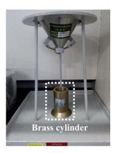
Fig. 1 Q/SY-2 bulk density meter.
