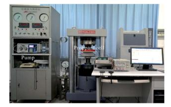
Fig. 6 Conductivity test device.
