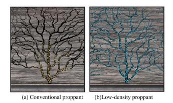
Fig. 11 Prop effect of conventional proppant and low-density proppant.<sup>28</sup>
