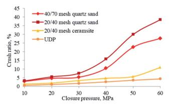
Fig. 16 Crushing ratio of different proppant at different closure pressures.
