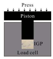
Fig. 4 Experimental device to test the compressive strength.
