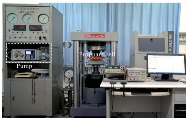
Fig. 6 Conductivity test device.
