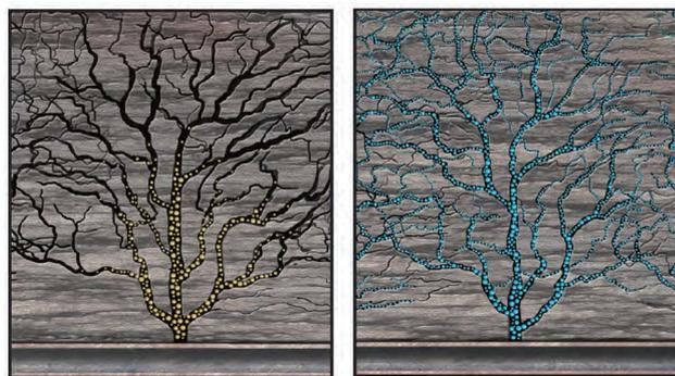
(a) Conventional proppant (b) Low-density proppant
