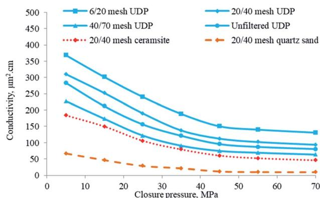
Fig. 20 Conductivity test results of different types of proppant.
