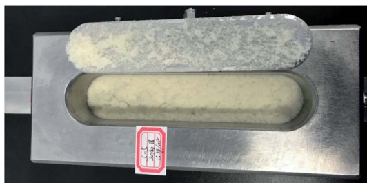
Fig. 5 Proppant cell in the conductivity test device.
