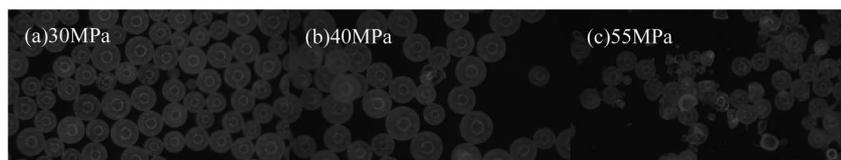
Fig. 17 Fragmentation of UDP at different closure pressures.
