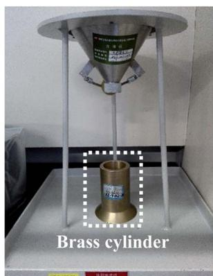
Fig. 1 Q/SY-2 bulk density meter.
