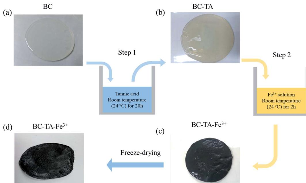
Fig. 1 Schematic of the BTF material fabrication. (a) BC sample, (b) BC-TA made by treating the BC with TA in step 1, (c) BC-TA-Fe<sup>3+</sup> (BTF), made by treating the BC-TA with Fe(III) solution in step 2, (d) BTF after freeze-drying.
