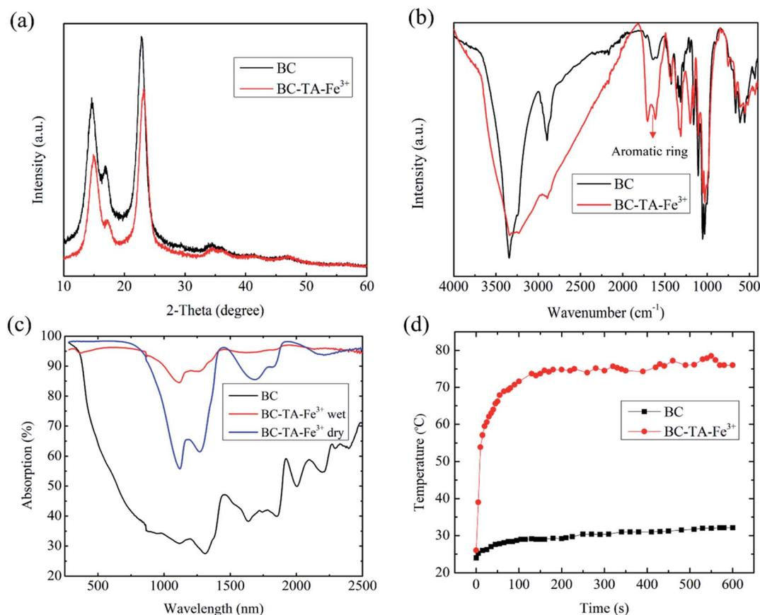
Fig. 3 (a) XRD patterns of BC and BTF materials showing slight changes in the diffraction peaks, (b) FTIR spectra of BC and BTF materials show peak height difference at around  $1610\text{ cm}^{-1}$ , (c) absorption spectra of the BC and BTF in dry/wet conditions in the wavelength range of 200–2500 nm, (d) the maximum temperatures of BC and BTF materials under 1 sun illumination recorded by an IR camera.
