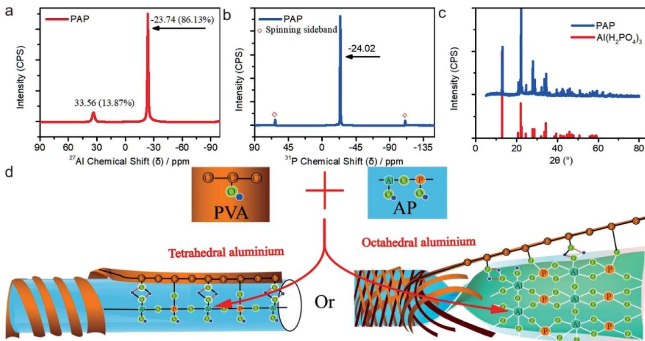
Fig. 4 (a)  $^{27}\text{Al}$  MAS NMR spectra; (b)  $^{31}\text{P}$  MAS NMR spectra; (c) XRD spectra of PAP and  $\text{Al}(\text{H}_2\text{PO}_4)_3$  (JCPDS no. 44-0724) and (d) possible structure of PAP.
