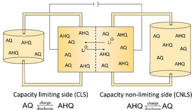
**Fig. 1** Schematic representation of an unbalanced compositionally symmetric redox flow cell setup utilizing anthraquinone (AQ) as well as anthrahydroquinone (AHQ) and the representative half-cell reactions in the capacity limiting side (CLS) and non-limiting side (CNLS).
