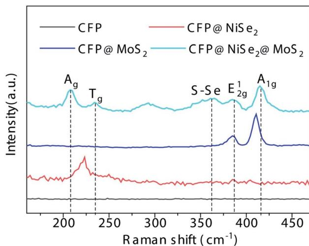
Fig. 3 Raman results of the samples. Peaks  $A_g$  and  $T_g$  belong to  $NiSe_2$ , while  $E_{2g}^1$  and  $A_{1g}$  belong to  $MoS_2$ . The presence of the peak S–Se confirms that the  $NiSe_2@MoS_2$  heterostructure was formed.
