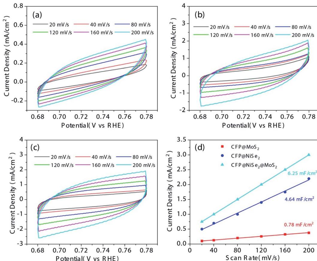
Fig. 7 CV tests of (a) CFP@MoS<sub>2</sub>, (b) CFP@NiSe<sub>2</sub>, and (c) CFP@NiSe<sub>2</sub>@MoS<sub>2</sub> with different scan rates from 20 to 200 mV s<sup>-1</sup> in a range of 0.68–0.78 V (vs. RHE). (d) Current density difference between anodic and cathodic versus the scanning rate at 0.73 V (vs. RHE).  $C_{dl}$  obtained by linear fitting the data was used to evaluate ECSA of the samples because  $C_{dl}$  was proportional to ECSA.
