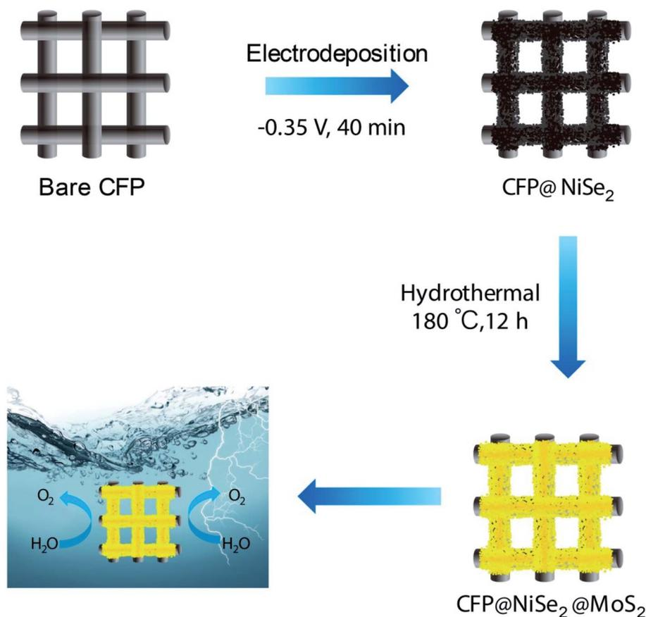
Fig. 1 Construction process of NiSe<sub>2</sub>@MoS<sub>2</sub> nano-heterostructures on CFP.
