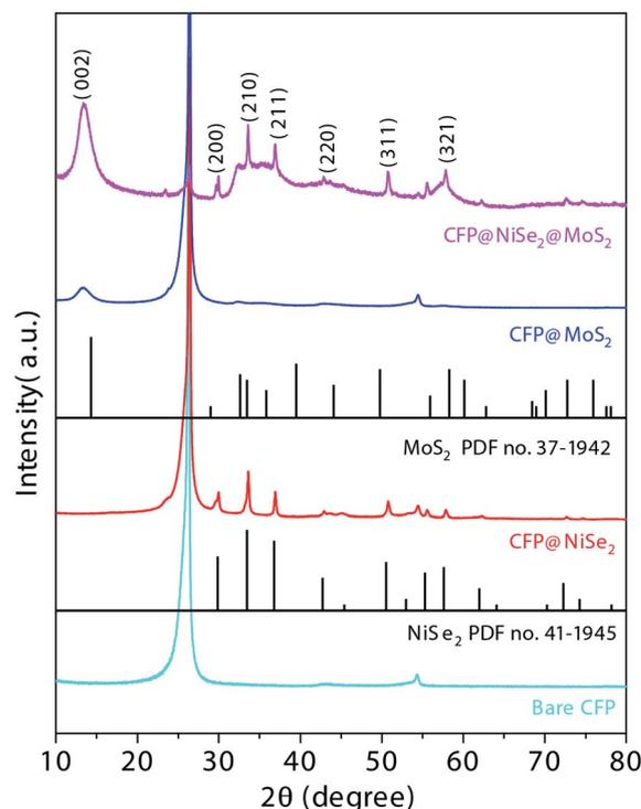
Fig. 4 XRD spectra of the samples. The standard diffraction peaks of  $NiSe_2$  and  $MoS_2$  are shown in PDF no. 41-1945 and no. 37-1942 respectively. Peaks (002) of  $MoS_2$ , (200), (210), (211), (220), (311), and (321) of  $NiSe_2$  are clearly exhibited.
