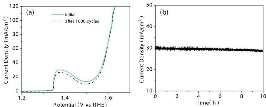
Fig. 8 (a) Durability measurement of CFP@NiSe<sub>2</sub>@MoS<sub>2</sub>. Difference in current density is negligible before and after 1000 cycles. (b) The current density versus time under a constant overpotential of 340 mV.
