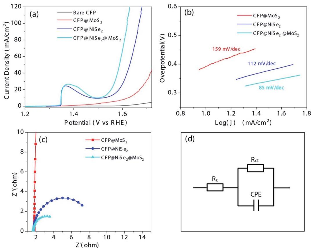
Fig. 6 (a) OER polarization curves, (b) Tafel plots, and (c) impedance analysis of the samples. (d) The equivalent circuit:  $R_s$  is the series resistance,  $R_{ct}$  is the charge-transfer resistance, and CPE is the constant phase elements.
