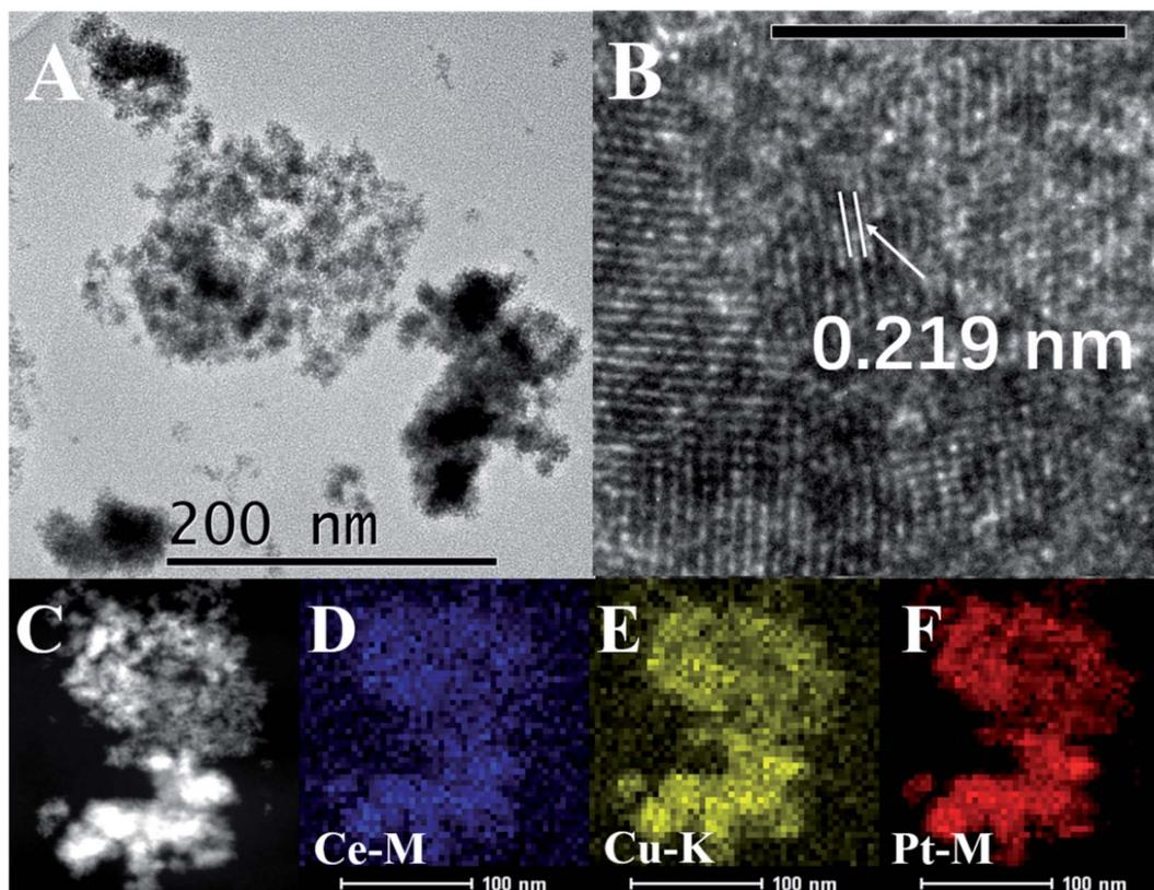
Fig. 2 TEM images of PtCu/CeO<sub>2</sub>-21 catalyst (A). The scale bar in the image (B) is 5 nm. Image (C) shows the area chosen for elemental mapping, image (D, E, and F) show the mapping of Ce, Cu, and Pt, respectively.
