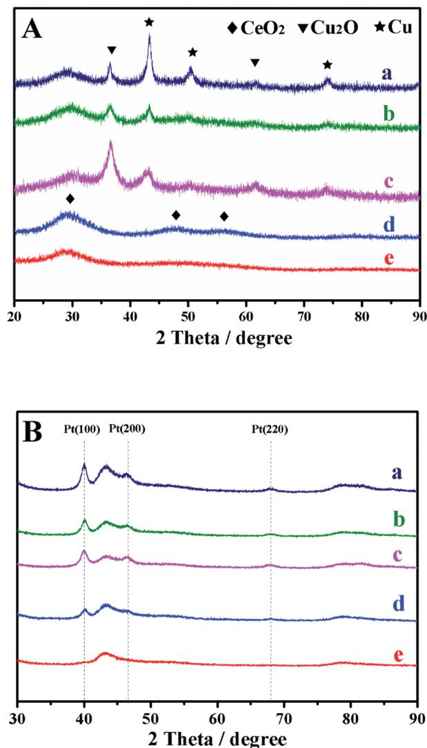
Fig. 1 XRD patterns of Cu–CeO<sub>2</sub> before (A) and after Pt deposition (B); (a), Cu–CeO<sub>2</sub>-31; (b), Cu–CeO<sub>2</sub>-21; (c), Cu–CeO<sub>2</sub>-11; (d), Cu–CeO<sub>2</sub>-12; (e), Cu–CeO<sub>2</sub>-13.
