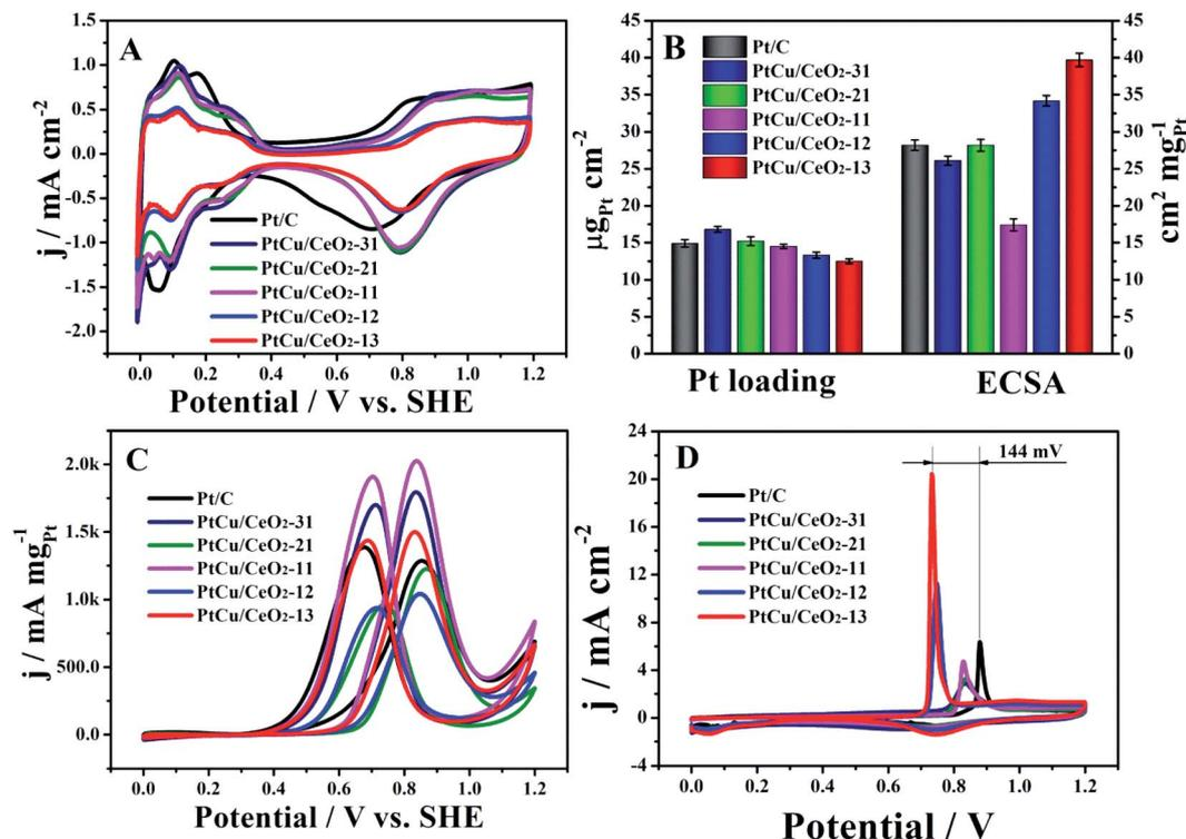
Fig. 4 (A): CVs of Pt/C and PtCu/CeO<sub>2</sub> catalysts in 0.5 M H<sub>2</sub>SO<sub>4</sub>; (B), Pt loading and ECSA values; (C), MOR mass activities of Pt/C and PtCu/CeO<sub>2</sub> catalysts in 0.5 M H<sub>2</sub>SO<sub>4</sub> and 1 M CH<sub>3</sub>OH; (D), CO stripping catalysts in 0.5 M H<sub>2</sub>SO<sub>4</sub>. The scan rate was 50 mV s<sup>-1</sup>.
