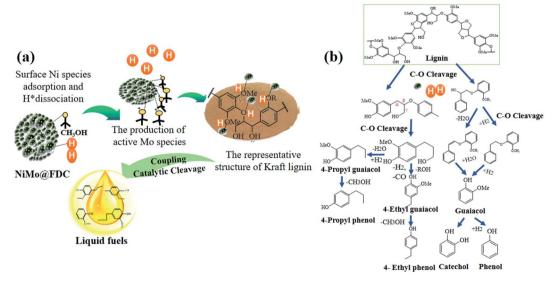
Fig. 10 Schematic diagram of possible catalytic depolymerization mechanism route.
