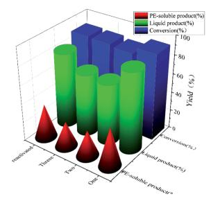
Fig. 9 Cycle experiments of 10%NiMo@FDC catalyst. Reaction conditions: 0.5 g of Kraft lignin, 0.2 g of catalyst, 25 mL of 1,4-dioxane and 5 mL of methanol, 300 °C, 12 h, 2 MPa H<sub>2</sub>.
