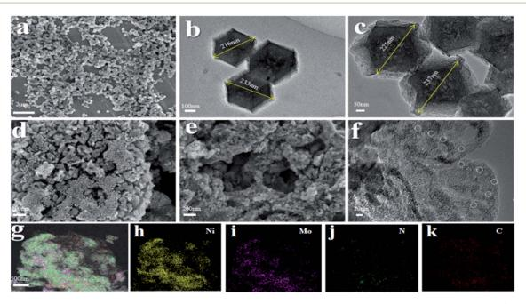
Fig. 2 SEM images (a), TEM images (b) of uncalcined precursor; TEM images (c) of ZIFs-derived carbon support; SEM images (d and e), TEM images (f), element mapping (g-k) of NiMo@FDC catalyst.
