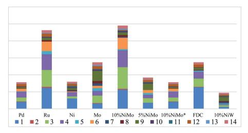
Fig. 7 The distribution of identified aromatic monomers in GC-FID analysis over various catalysts. Reaction conditions: 0.5 g of Kraft lignin, 0.2 g of catalyst, 25 mL of 1,4-dioxane and 5 mL of methanol, 300  $^{\circ}$ C, 3 h, 2 MPa H<sub>2</sub>.
