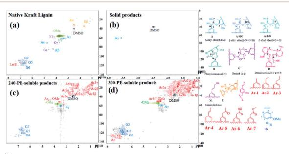
Fig. 8  $^{1}$ H $^{-13}$ C HSQC NMR spectra of lignin and PE-soluble products obtained after catalytic depolymerization using 10%NiMo@FDC catalyst at 300  $^{\circ}$ C, 2 MPa H $_{2}$  and 12 h; (a) Native Kraft Lignin, (b) solid product; (c and d) PE-soluble products.
